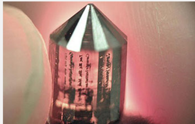
Five-carat diamond laser-cut from a 10-carat single crystal produced by high-growth rate CVD Credit and Larger Version
