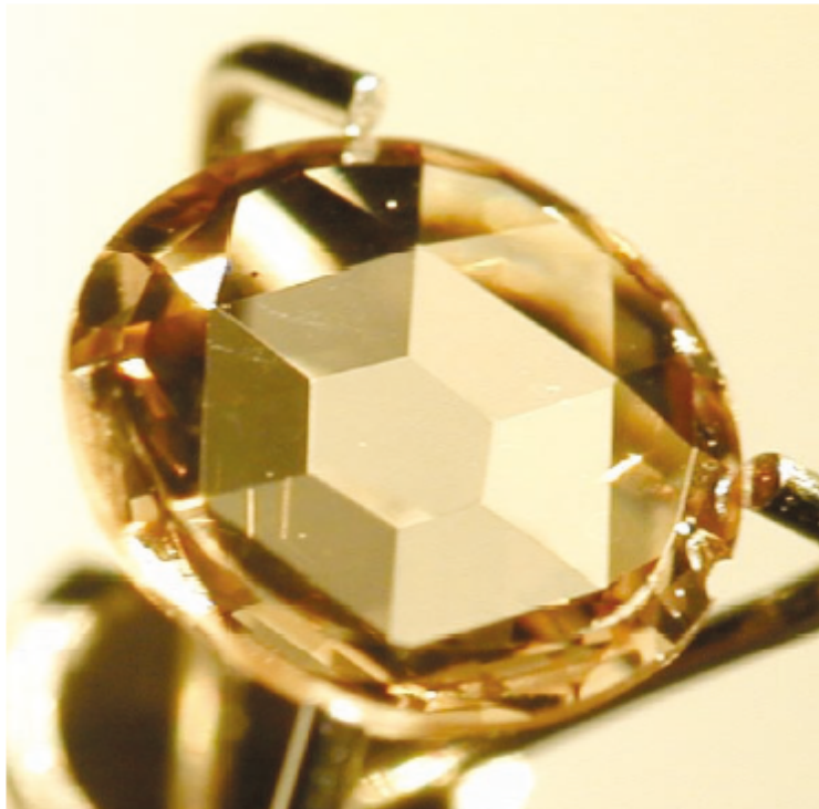
Fig. 1. Photographs of single crystal diamond grown by chemical vapor deposition (CVD) (Courtesy of Apollo Diamond): (a) a faceted stone ca. 3 mm diameter, in which single qubit operations for quantum computing have been demonstrated at room temperature using the N-V defect; and (b) a homoepitaxial layer ca. 4 x 4 x 1 mm (white/clear) after separation from the adjacent to the original HPHT seed crystal (yellow).
