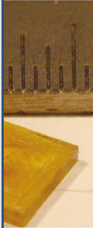
The CVD process can produce a variety of single crystal diamonds. Credit and Larger Version
