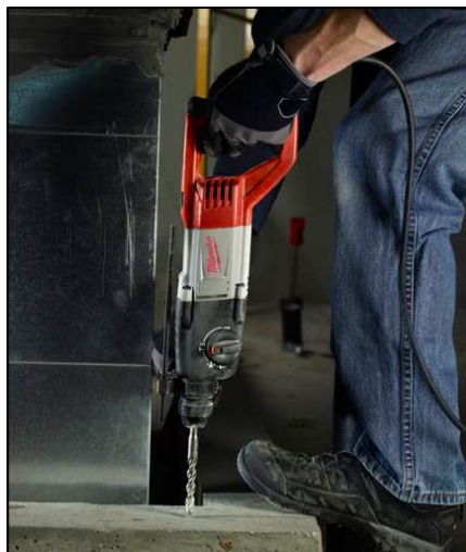
Figure 1-10 – 5262-20 rotary hammer in a typical drilling application (6)
