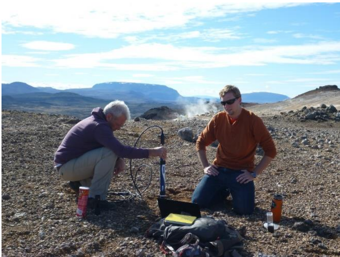
Figure 7- Author and co-advisor using a Hydrolab sonde in the field.
