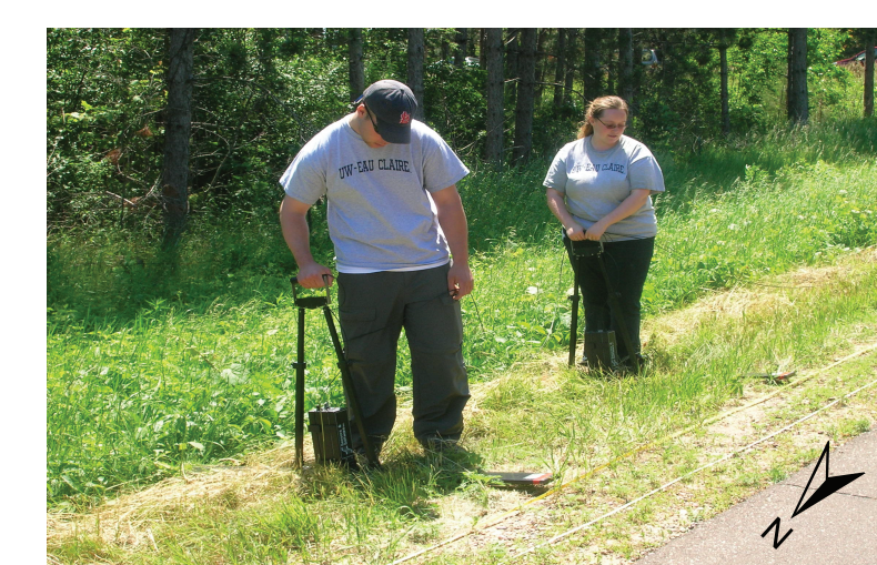
Figure 3b: Common midpoint data collection on Wissota Terrace along 1000th St. (R1). View to the southeast.
