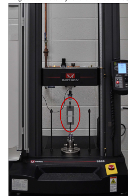
Our tensile tester. Test set-up highlighted.
