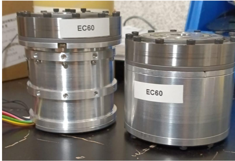
Figure 42: Final and initial version of the custom integrated actuator.
