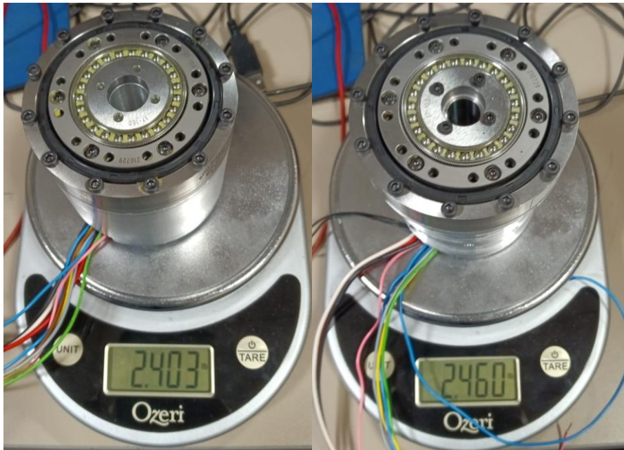
Figure 32: Actuators weight, initial and final version.
