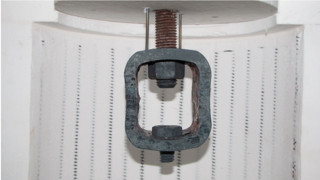
Figure 5-4 Failure in top section of the specimen (Test02 – First Group)
