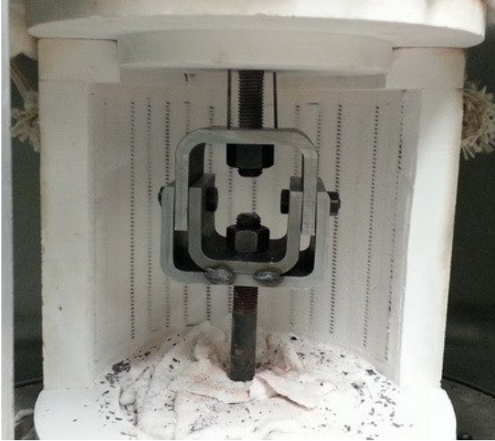
Figure 5-41 A shear test specimen
