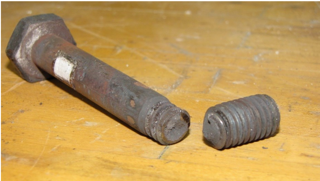
Figure 3-12 Failure in the threaded section
