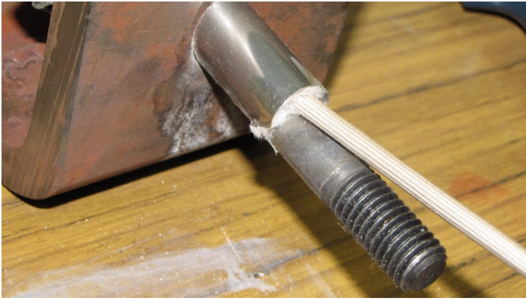
Figure 3-5 Strain gage covered with ceramic fiber and a protective cover
