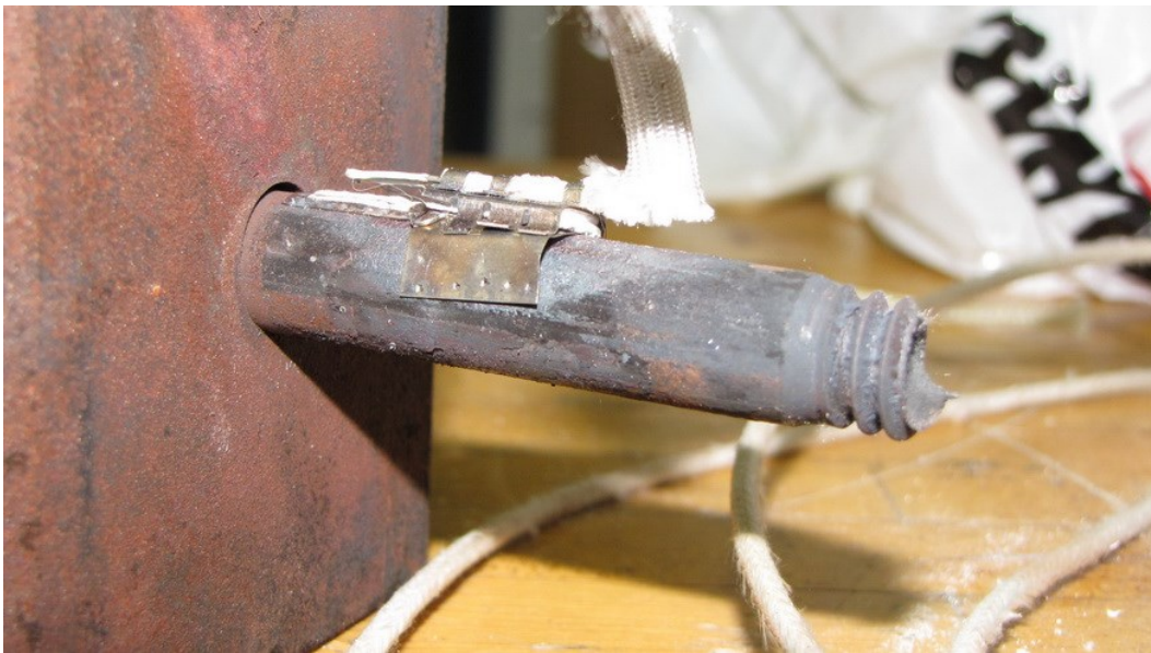
Figure 3-15 A close up look at the strain gage after the test
