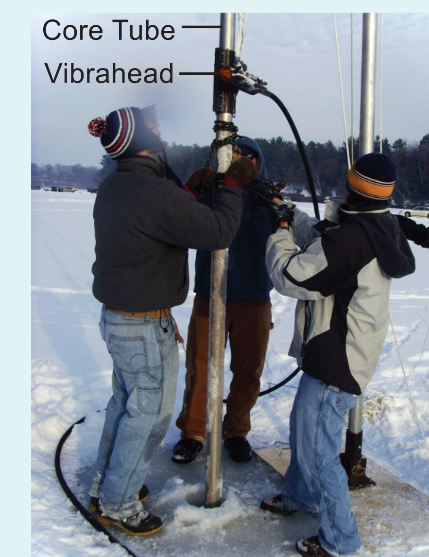
Figure 5: The vibrahead and core tube are visible while coring HML-4
