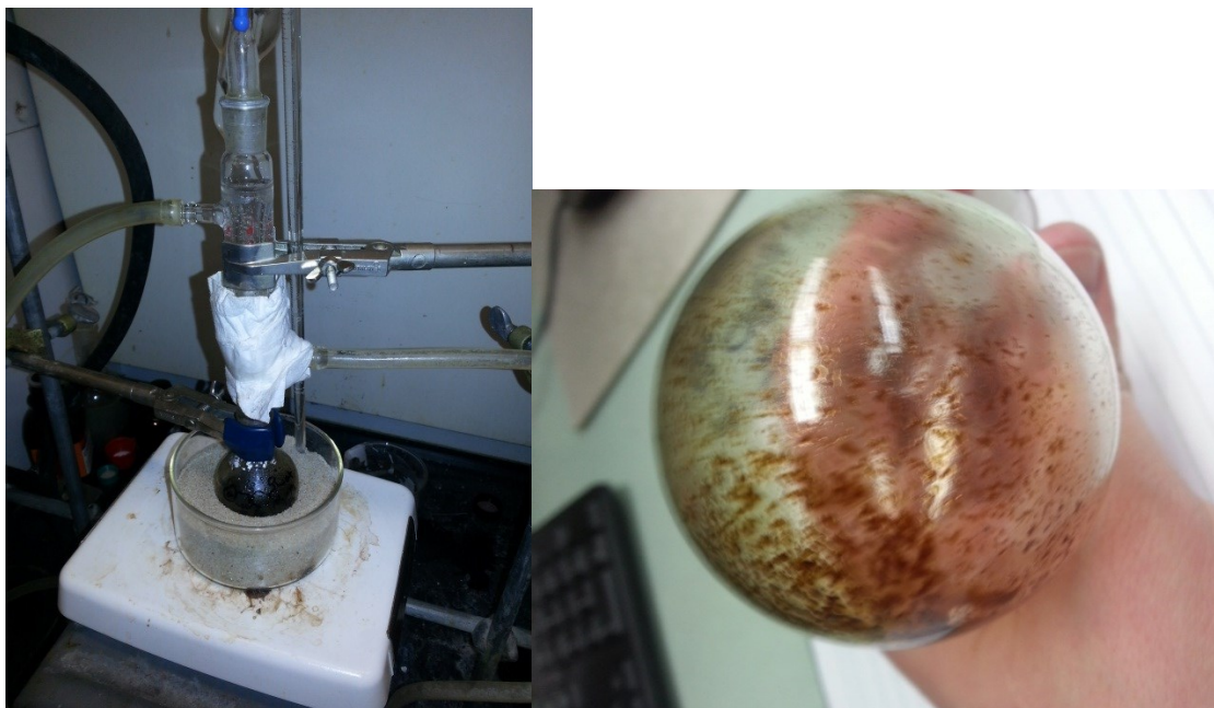
Figure 42. Charred reaction product
