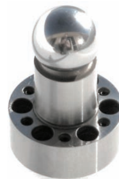
Fig. 9. Monolithic Ø19 mm flange-mounted ball. The superior stiffness of the screw joint flange-mount and single-piece ball is essential for nanometer-level error motion measurement at high speeds.
