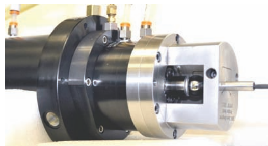
Fig. 8. Tooling for radial and axial error motion measurement is designed to minimize structural error motion.
