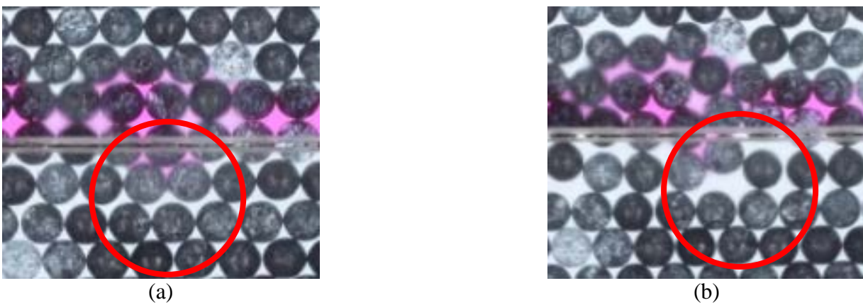
Figure 6.12 Zoomed in images of wet 1.0 mm/min Glass beads inclined at 18° (a) prior to vertical movement in circled region and (b) after vertical movement in circle region
