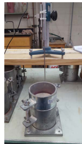
Figure 4.4 Apparatus on elevated platform; sample prior to final lift of material
