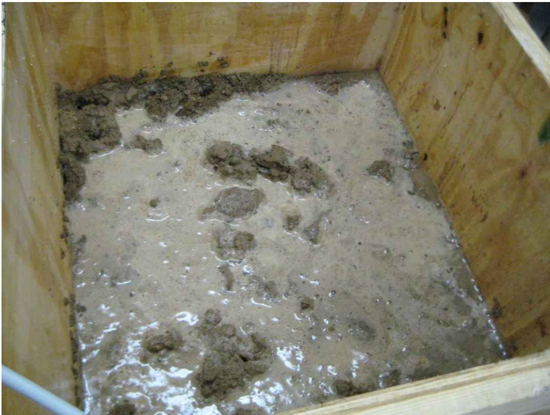
Figure 4.15. Silty Sand in Viscous State Upon Completion of Jetting.
