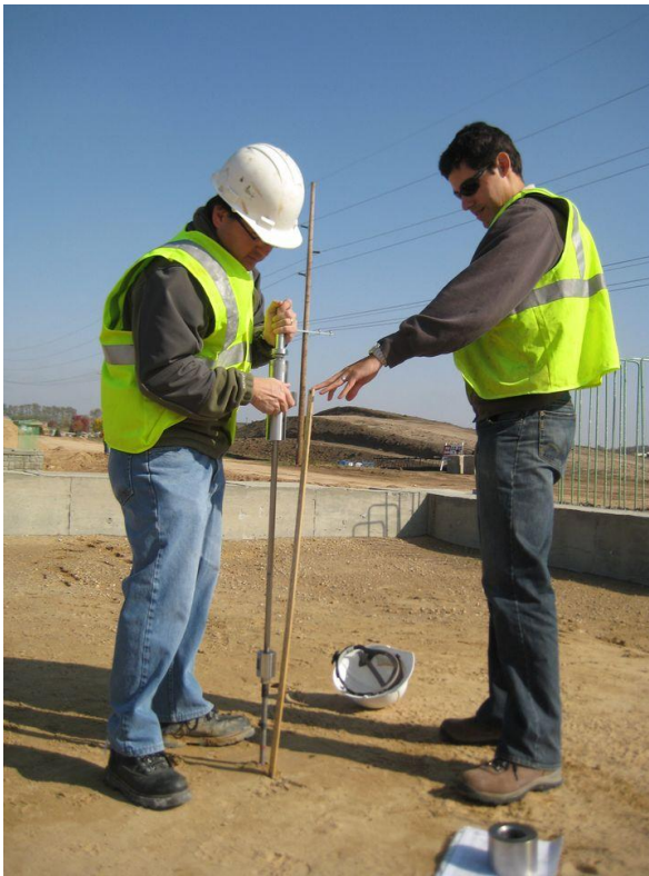
Figure 5.5. DCP in Action (left). Close-up of Fissured Flooded-Compacted Backfill (right).
