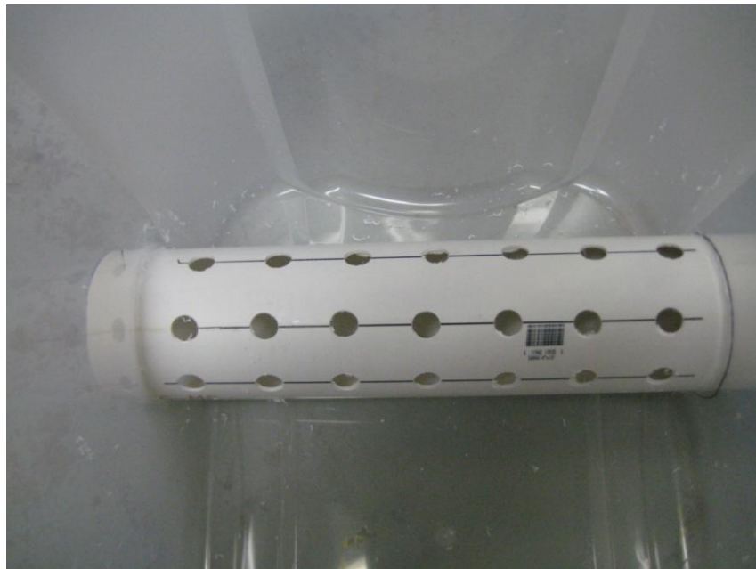
Figure 4.11. Drain Tile Constructed from PVC Pipe (top).
