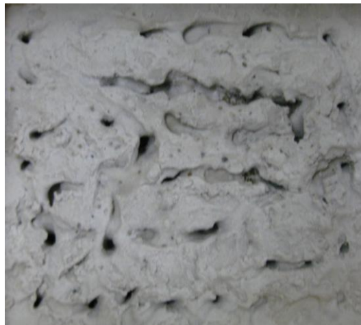
Figure 4.12. Voids Left Over After Jetting a Regular Grid. 100% silica sand soil is shown here.
