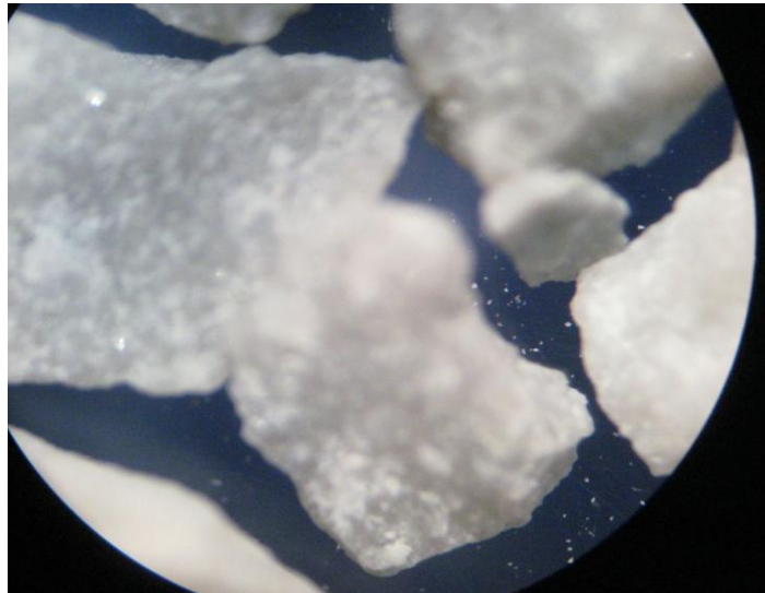
Figure 3.5. Microscope Image of Limestone Screenings.
