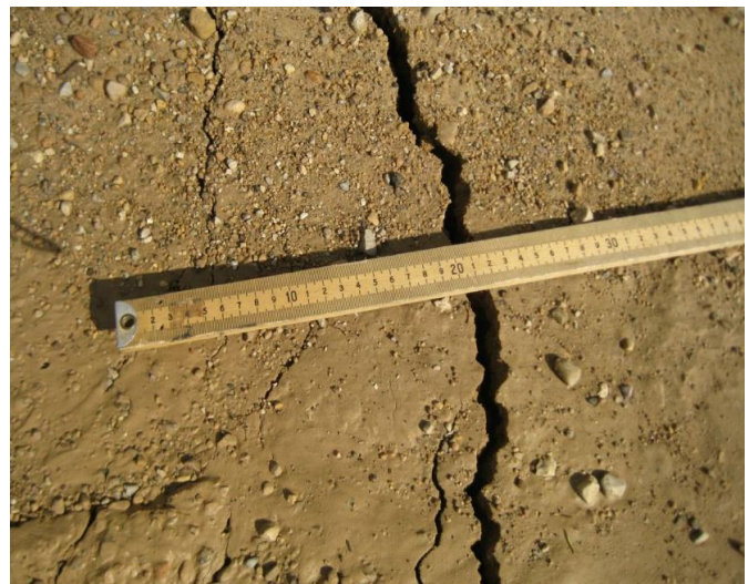
Figure 5.5. DCP in Action (left). Close-up of Fissured Flooded-Compacted Backfill (right).
