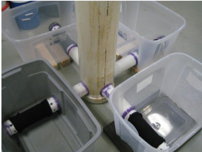
Figure 4.11. Setup with Central Drainage Column (bottom). The PVC pipes were angled downward into the central drainage column; water flowed into the column and out of additional hoses connected to the base of the column. The tubs shown in the bottom image were filled to the top with the soils and jetted.
