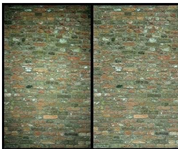
Figure 4.4 Vignetting seen in a photograph for two aperture sizes. Left: f/1.4 . Right: f/5.6 [29].
