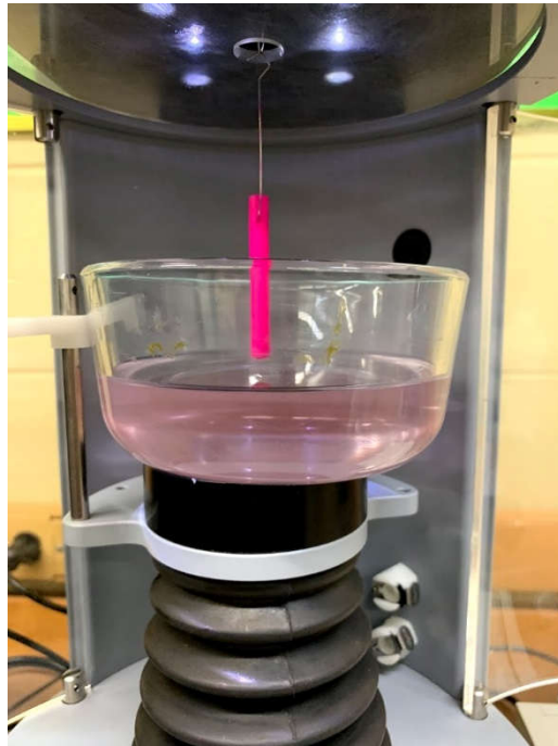
Figure 12. The tensiometer (also called DCA or the dynamic contact angle analyzer) used for measuring the contact angle
