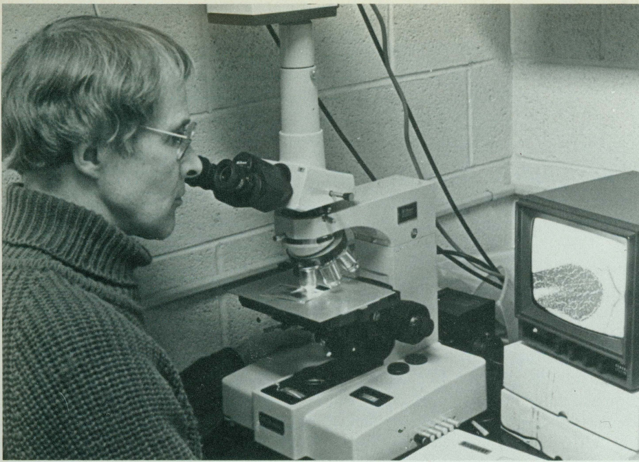
Professor of Neurophysiology Wally Welker examines a slide from the Department's extensive brain collection. A stained section is projected on a video screen (right) where, in conjunction with a computer, features can be quantified and measured in great detail.
