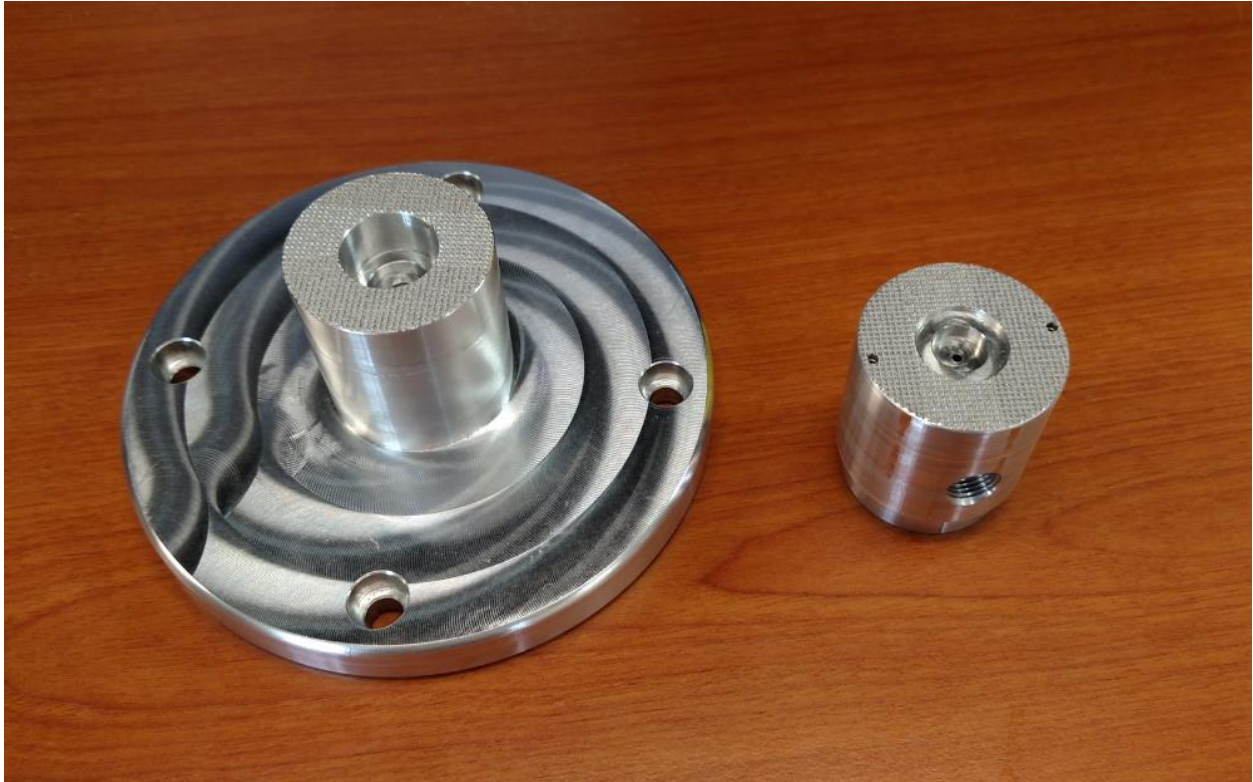
Figure E-3: Resonant column suction control components.
