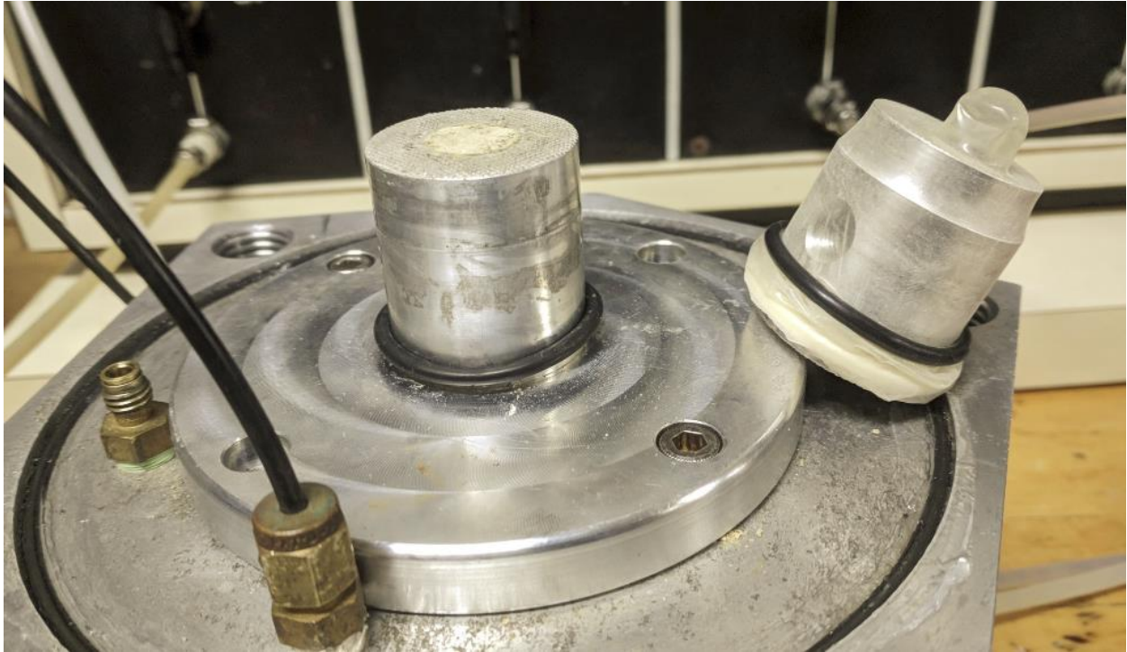
Figure 2.2: Top and bottom platen with O-rings and membrane prepped.
