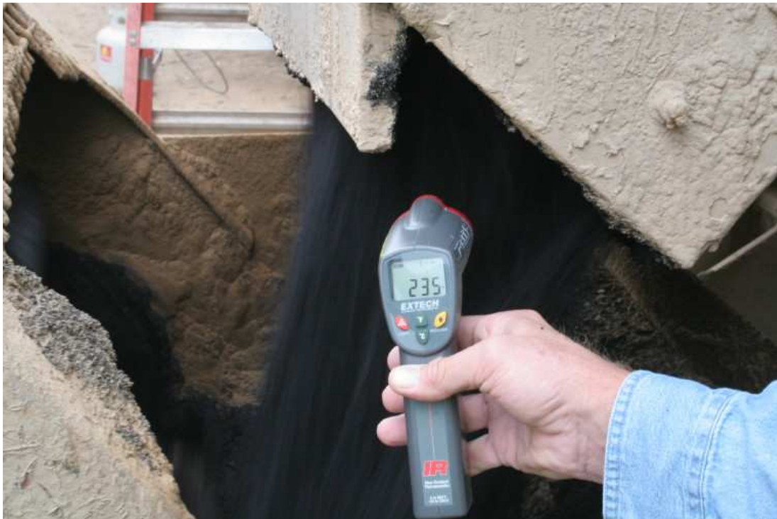
Figure 6.5 Warm Mix Temperature Reading at Drum Discharge
