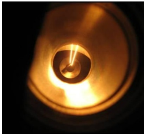
Figure A-1: Photo taken through view-port of tungsten wire recrystallization. The circular object in the center is a 2 kg weight which keeps the wire under considerable tension. (image used with permission Boscoboinik)
