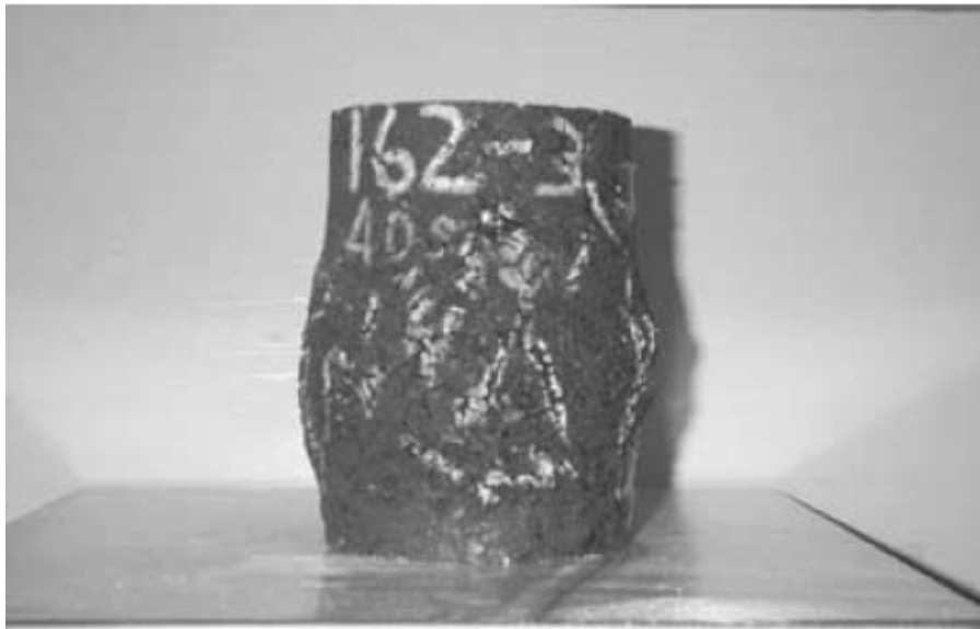
Figure 2-7: Observed macro-cracking on an asphalt mixture sample [24]
