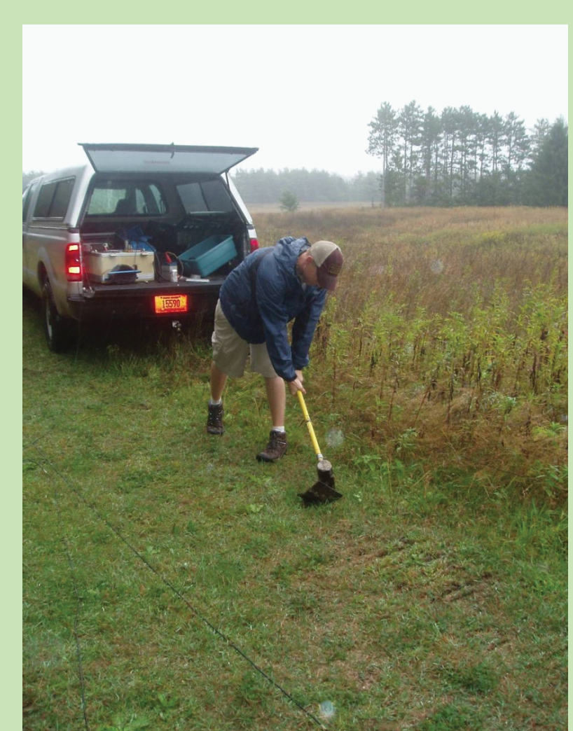
Figure 8: A metal plate was struck with a sledgehammer to create a seismic wave.
