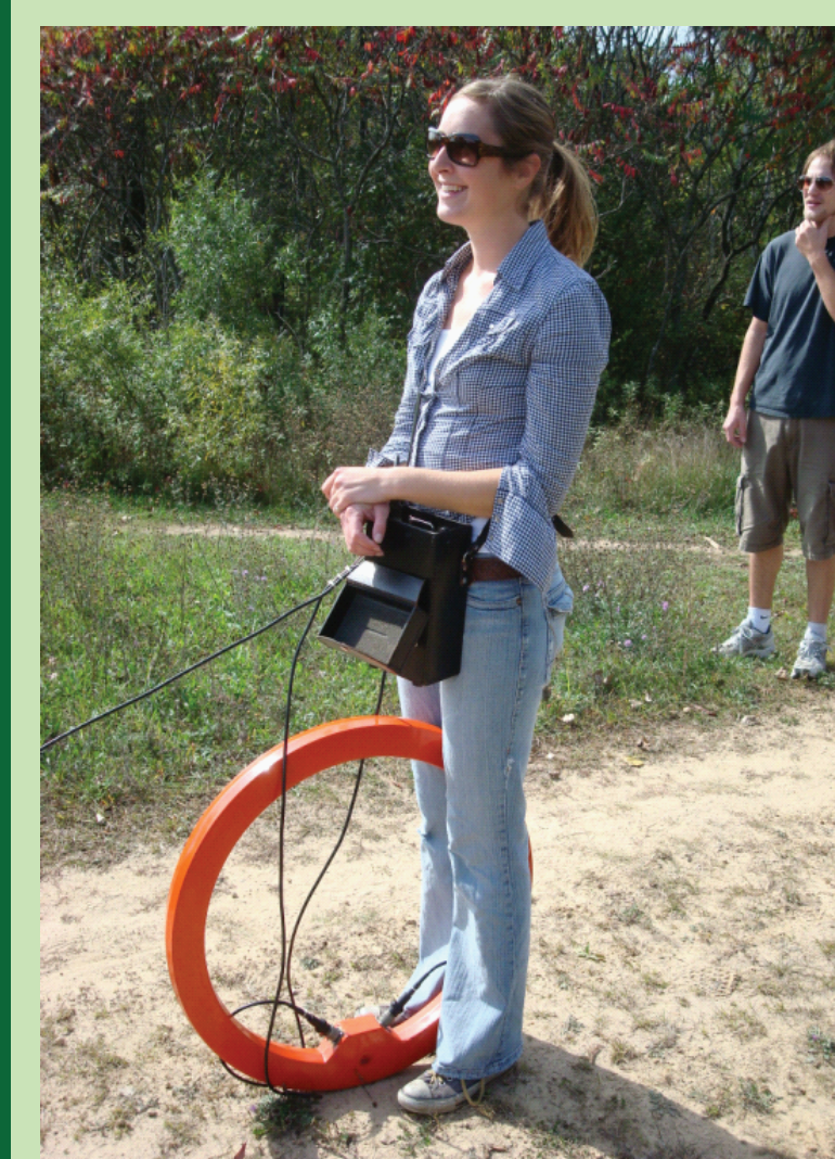
Figure 6: A Geonics EM 34 was used to acquire electrical conductivity data.
