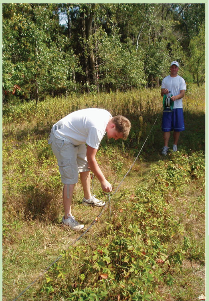
Figure 3: An Offset Wenner array was used to acquire resistivity measurements.
