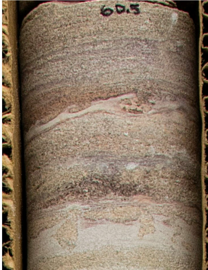
Figure 30. Buchda Quarry, Box 40. Tunnel City Tomah Member millimeter-to centimeter- scale flame structures.
