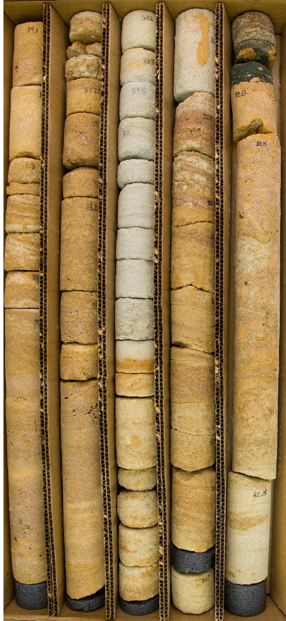
Figure 33. Alsum 4, Box 25. Mazomanie Formation cross-stratified sandstone facies and bioturbated sandstone facies overlain (top right corner) by a glauconitic sandstone bed with centimeter-scale Mazomanie sandstone rip-up clasts.
