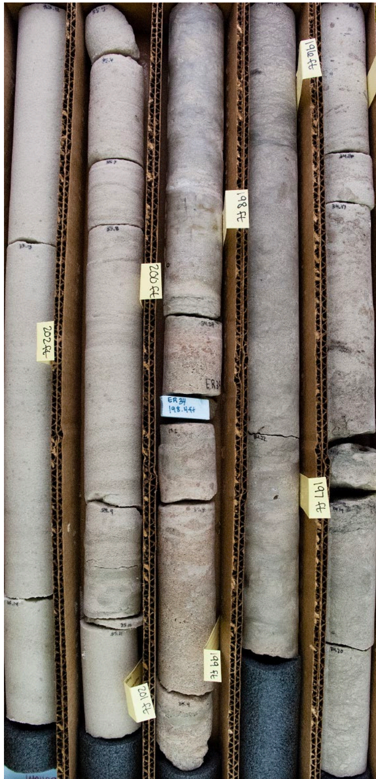
Figure 34. Bleeker, Box 21. Saint Lawrence Formation sandy dolomite facies with bioturbation and burrows.
