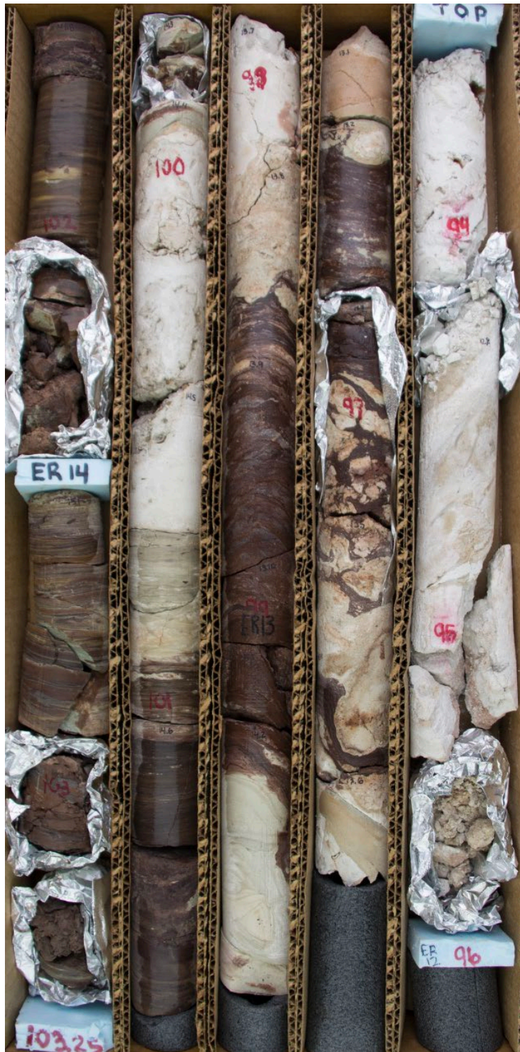
Figure 42. Slinger, Box 6. Deformed horizon in the upper Prairie du Chien with angular reworked dolomite clasts, soft-sediment deformation, silcrete accumulation, and poor consolidation.
