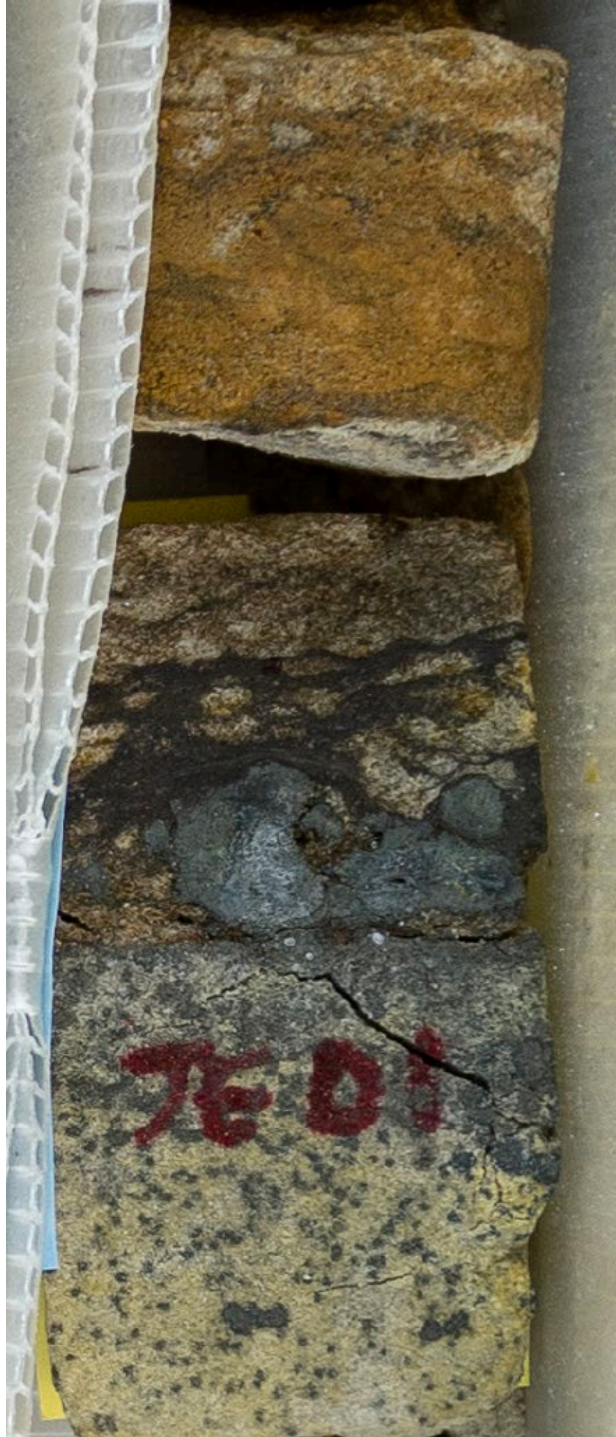
Figure 86. Mobil, Box 27. Abrupt Saint Peter- Sinnipee contact with abundant millimeter- to centimeter-scale sulfide mineralization.
