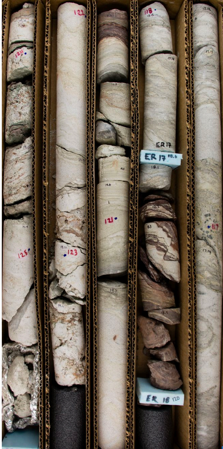
Figure 43. Miller Quarry, Box 12. Deformed lower Readstown Member with brecciated clasts, silcrete accumulation, brittle offset and minor fracturing, and soft sediment deformation.
