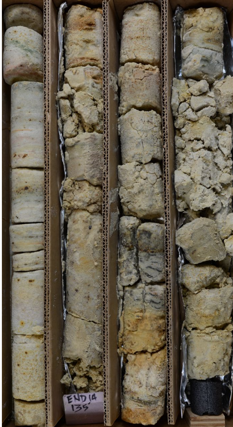
Figure 83. HBFA, Box 16. Saint Peter Tonti Member cross-stratified sandstone facies with weak cementation, bioturbation, and sulfide mineralization.
