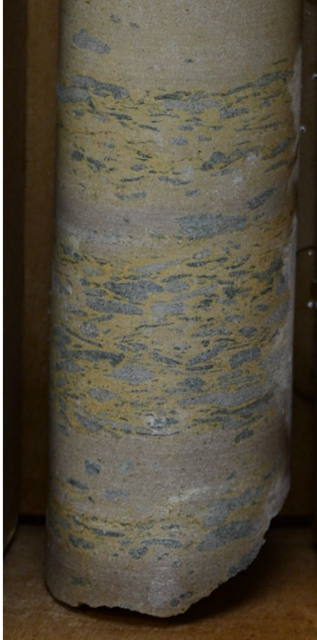
Figure 77. HBFA, Box 31. Saint Lawrence dolomite with horizontal sand-filled burrows in silty dolomite beds.
