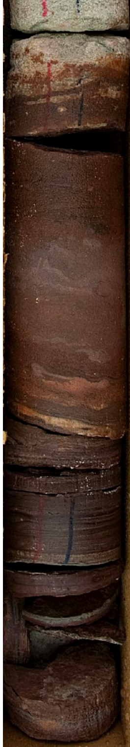
Figure 57. Highway T, Box 34. Oxidized sand and mud of Jordan Formation, possible paleosol.
