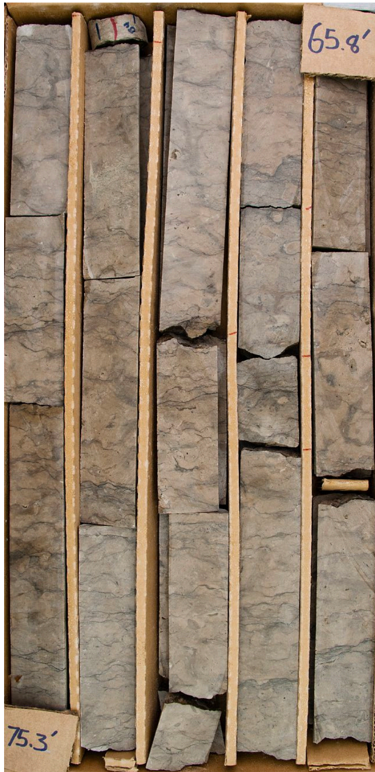
Figure 49. Swan Road, Box 6. Decorah Formation dolomite mudstone facies with wispy shale partings.
