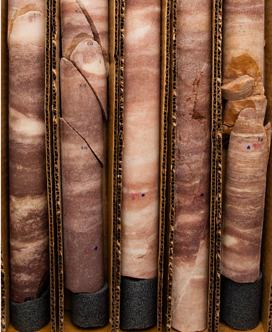
Figure 14. Salna. Box 4. Mazomanie Formation cross-bedded sandstone.
