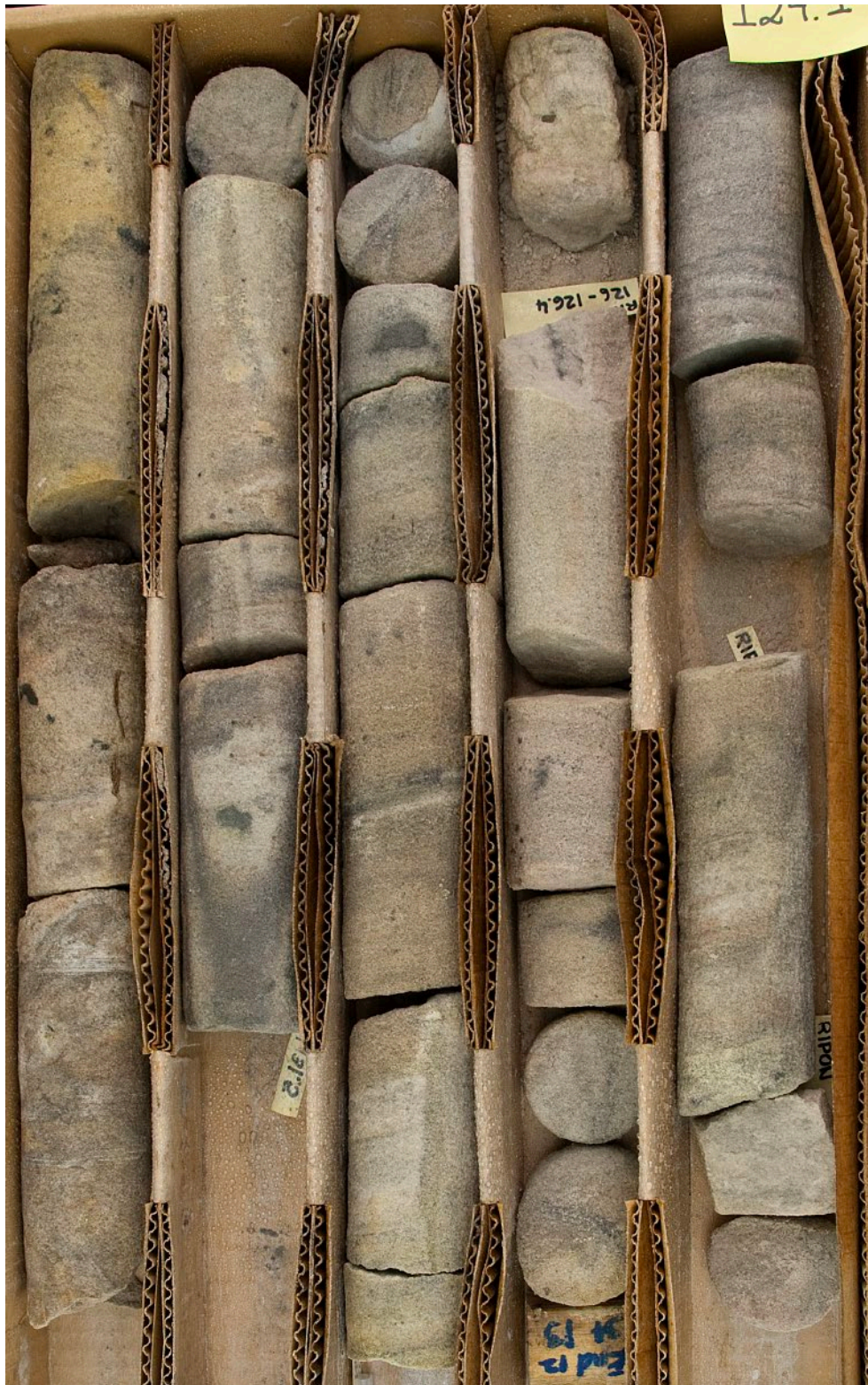
Figure 67. Ripon, Box 12. Upper Tonti Member cross-stratified sandstone facies with brittle offset, sulfide mineralization, and burrows.
