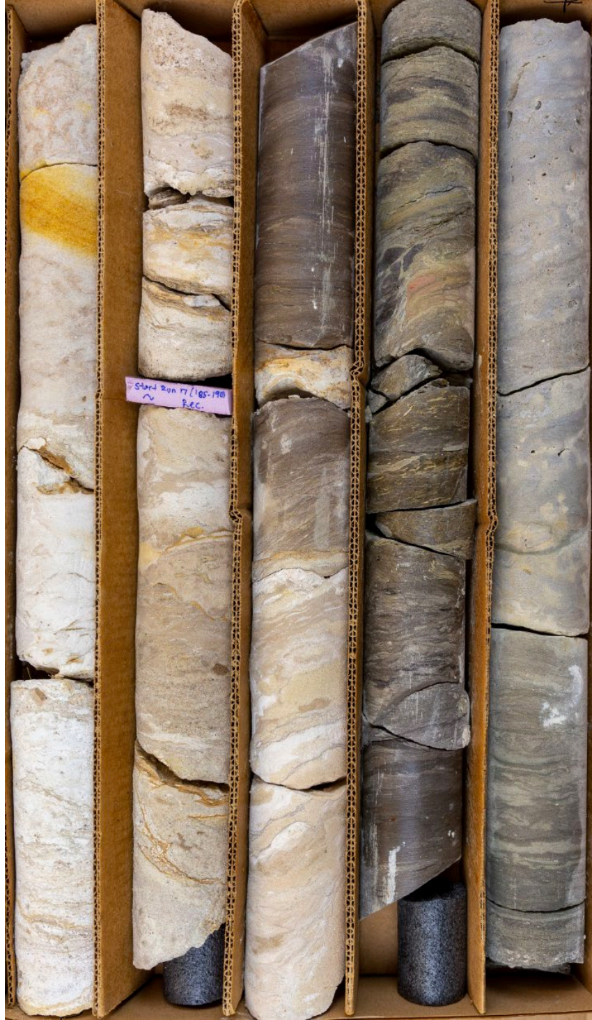
Figure 79. Mankowski, Box 16. Jordan-Prairie du Chien contact with silcrete accumulation, reworked bedding, and brecciated reworked clasts.
