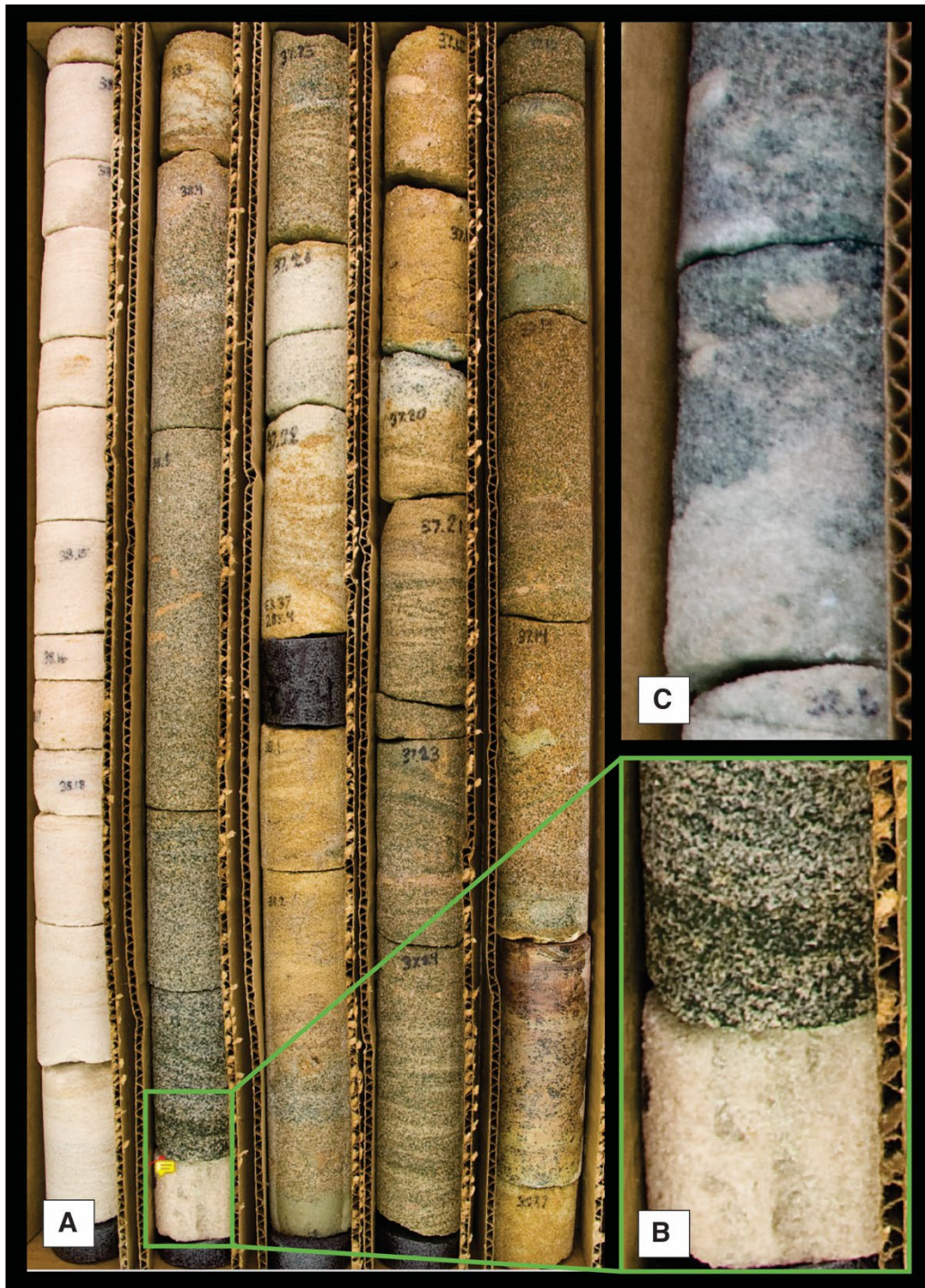
Figure 28. Wonewoc-Tunnel City contact. (A, B) Alsum 4, Box 29. Sharp contact between Wonewoc clean sandstone (bottom), and Tunnel City glauconitic sandstone (top). Lower strata in bottom left, upper strata in top right. (C) Slinger, Box 22. Erosional contact with millimeter-to centimeter-scale Wonewoc rip-up clasts.
