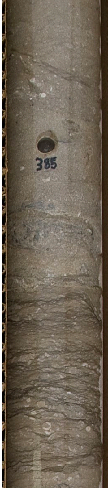
Figure 51. Neda, Box 37. Galena Formation fossiliferous to fine-grained dolomite parasequence.
