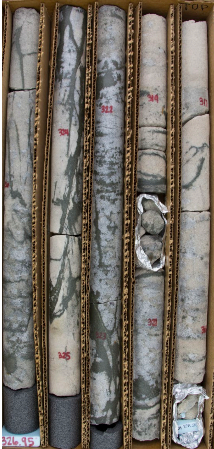
Figure 26. Slinger, Box 30. Wonewoc Formation fractured sandstone facies with abundant sulfide mineralization.
