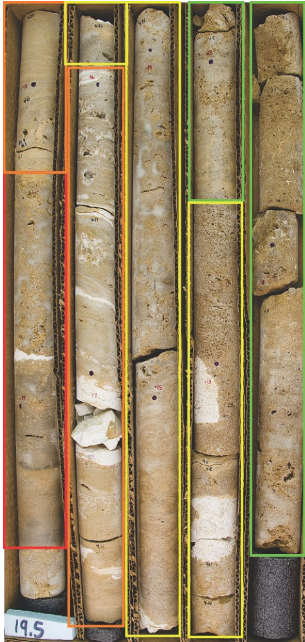
Figure 19. Arlington Quarry, Box 2. Prairie du Chien coarsening upwards parasequences. Lower strata in bottom left, upper strata in top right. Each parasequence outlined in a different color.
