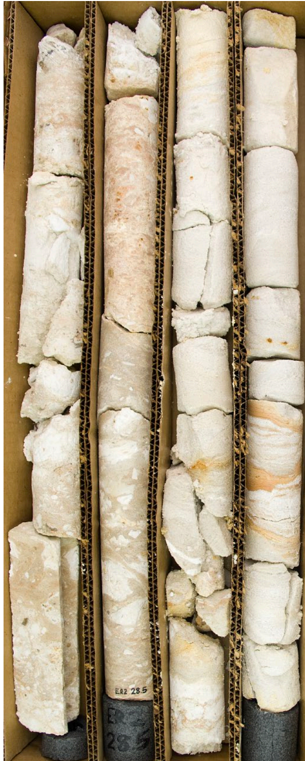
Figure 21. Columbus 2, Box 1. Saint Peter Formation Readstown Member lower brecciated silicified sandstone facies (left) and upper massive sandstone facies (right).
