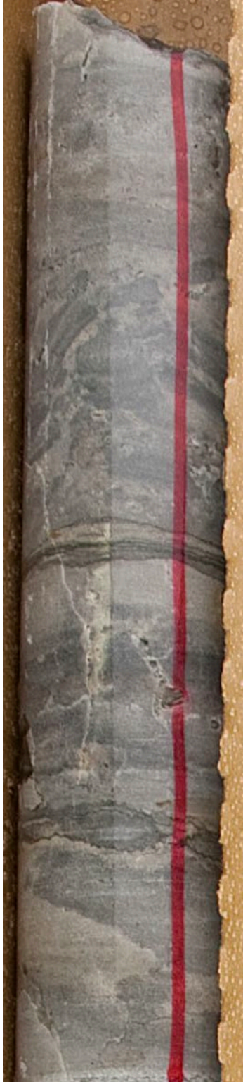
Figure 61. Highway T, Box 22. Prairie du Chien karst-mottled dolomite with dolomite breccia.
