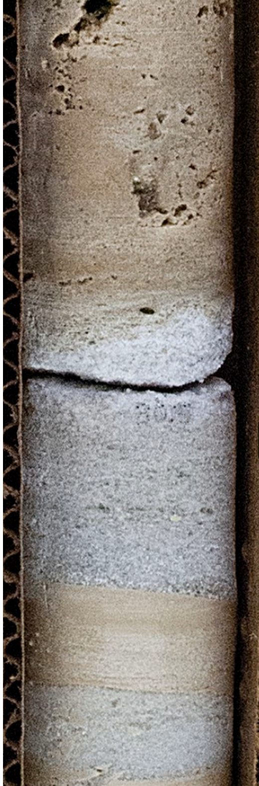
Figure 38. Bleeker, Box 16. Lower Prairie du Chien Oneota coarse, silcretic sandstone “bubble rock”.
