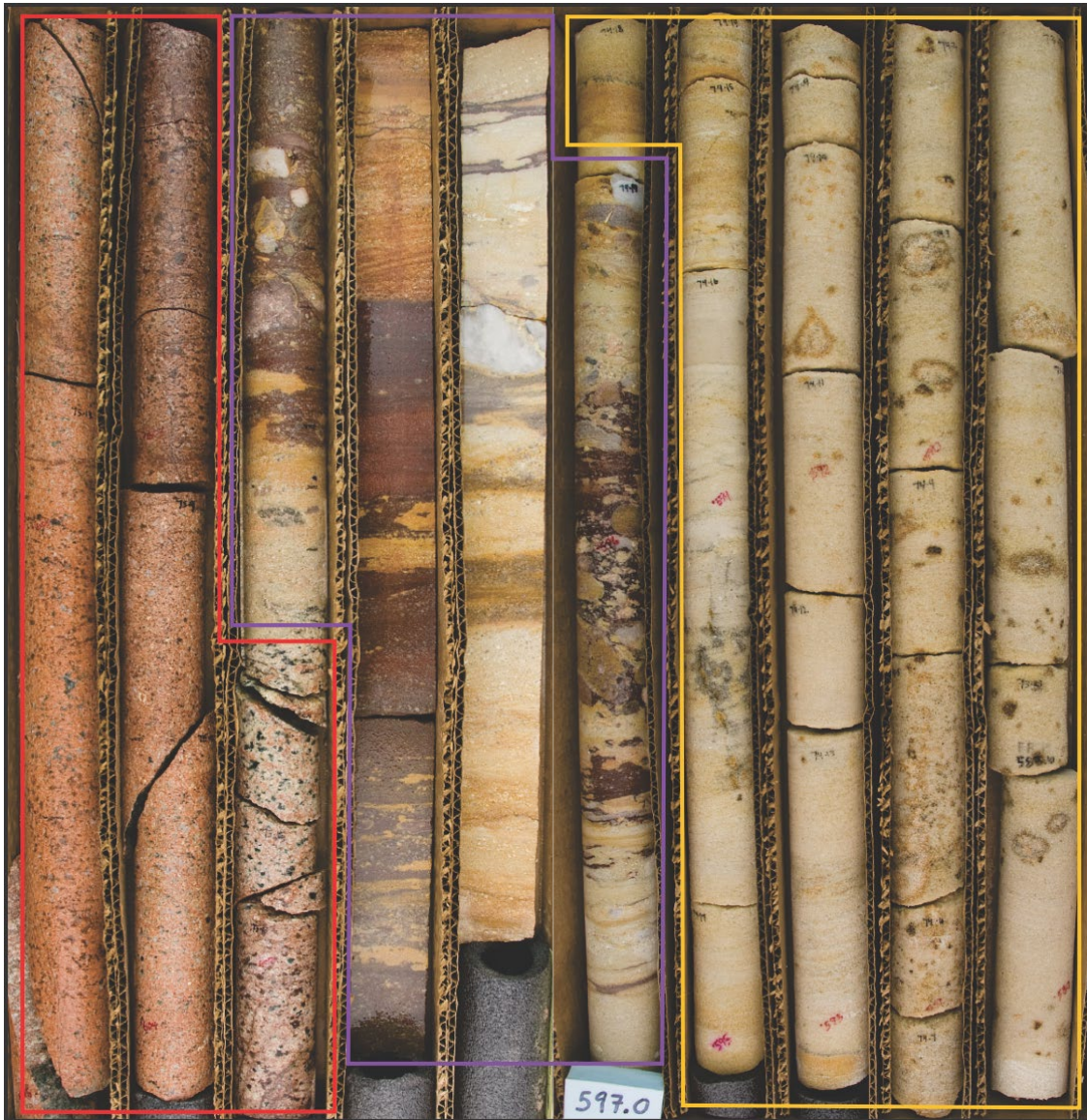
Figure 5. Triemstra core, Box 58 and 59. Transition from Precambrian granite (bottom left) to Mount Simon sandstone (top right). Precambrian is outlined in red, conglomerate is outlined in purple, and Mount Simon sandstone is outlined in yellow.
