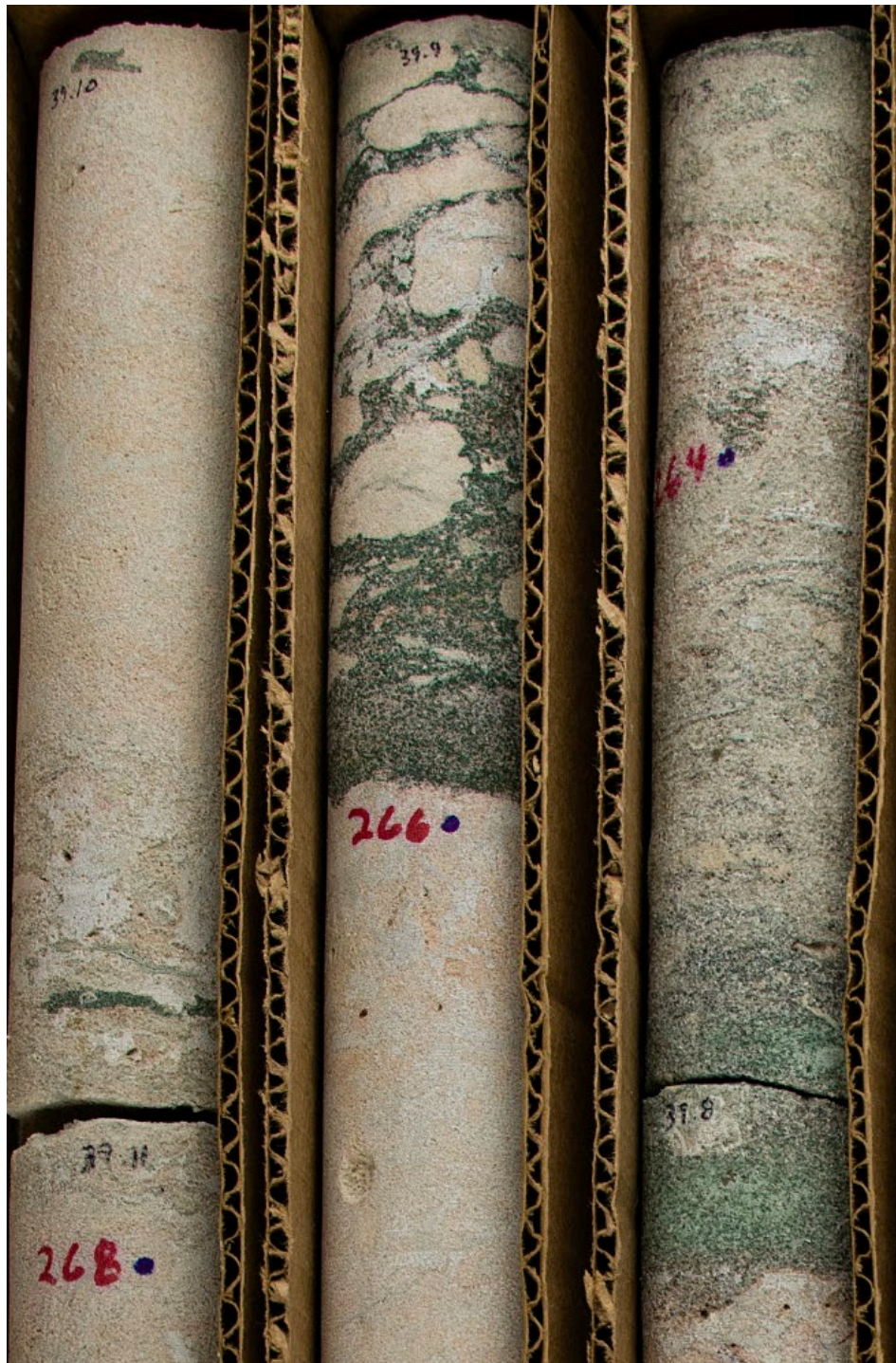
Figure 32. Miller Quarry, Box 28. Tunnel City Reno Member (above and to the right of marker “266”) with centimeter-scale rip-up clasts of underlying Tomah “wormstone” (below and to the left of marker “266”) in glauconite sand.
