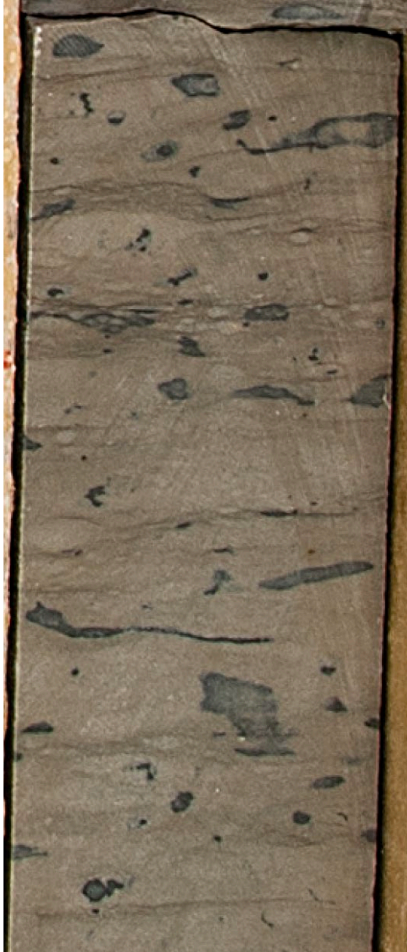
Figure 48. Swan Road, Box 20. Platteville Formation muddy dolomite facies with mud-lined burrows.
