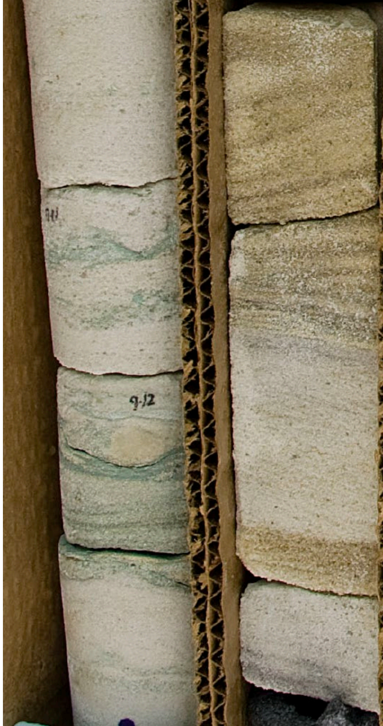
Figure 16. Arlington Quarry, Box 5. Jordan Formation shaly sandstone facies (left) and cross-bedded sandstone facies (right).
