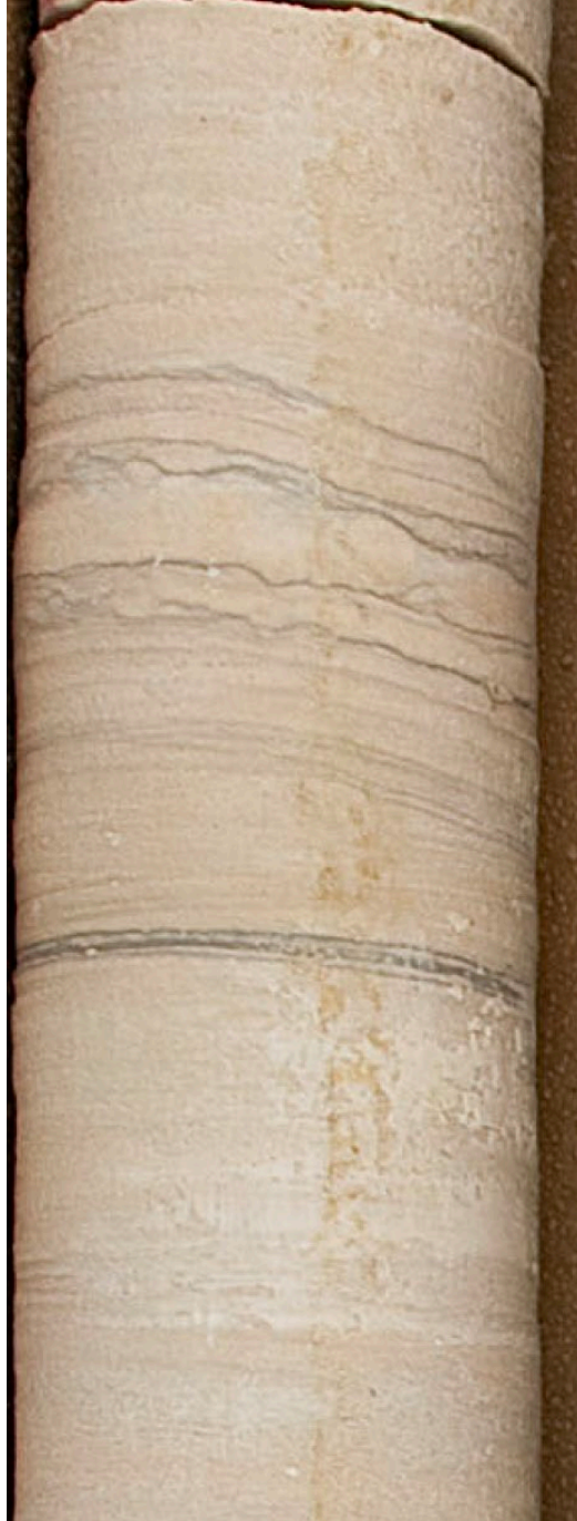
Figure 55. Rosendale, Box 31. Trempealeau Group Saint Lawrence Formation silty dolomite with shale partings.
