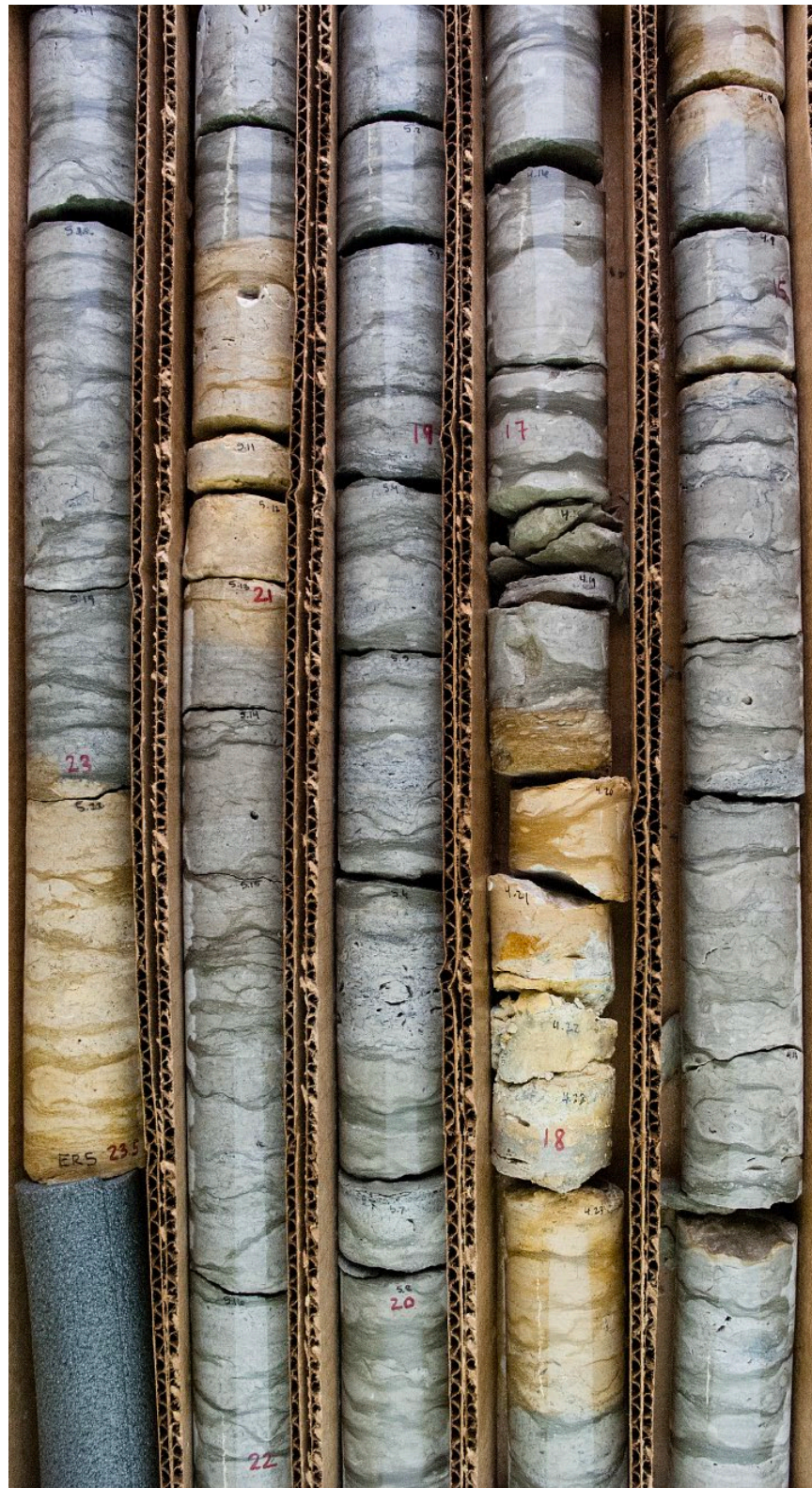
Figure 47. Bleeker, Box 2. Platteville Formation dolomite wackestone with shale partings.
