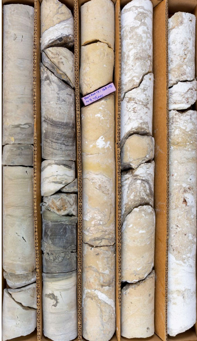
Figure 81. Mankowski, Box 14. Prairie du Chien- Saint Peter deformed contact with silcrete accumulation, brecciated reworked dolomite and silcrete clasts, rip-up clasts, and brittle offset.
