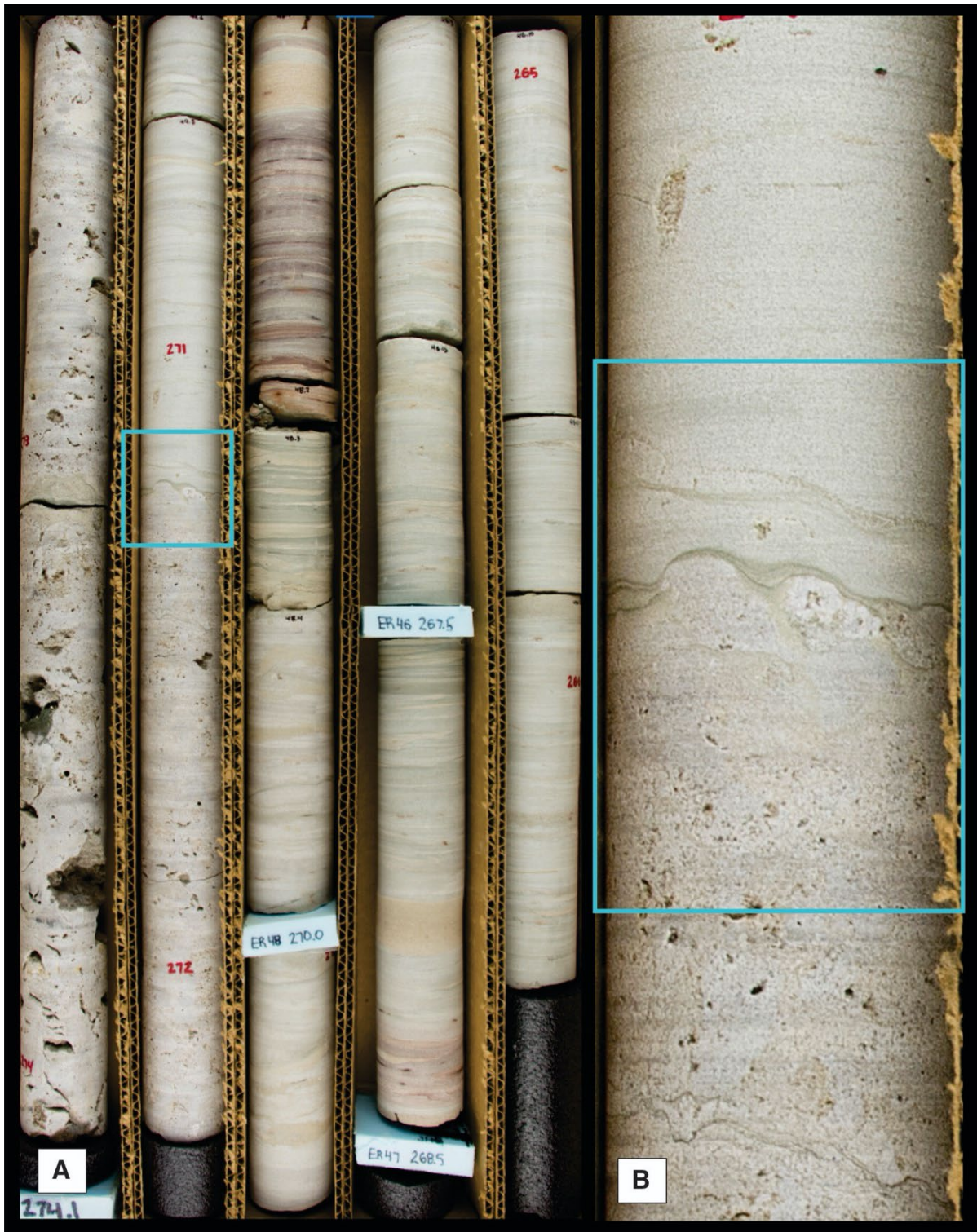
Figure 39. (A) Buchda Quarry, Box 30. Porous, vuggy Oneota Formation (bottom left) and laminated, silty Shakopee Formation (top right). (B) Enlarged sharp contact horizon.
