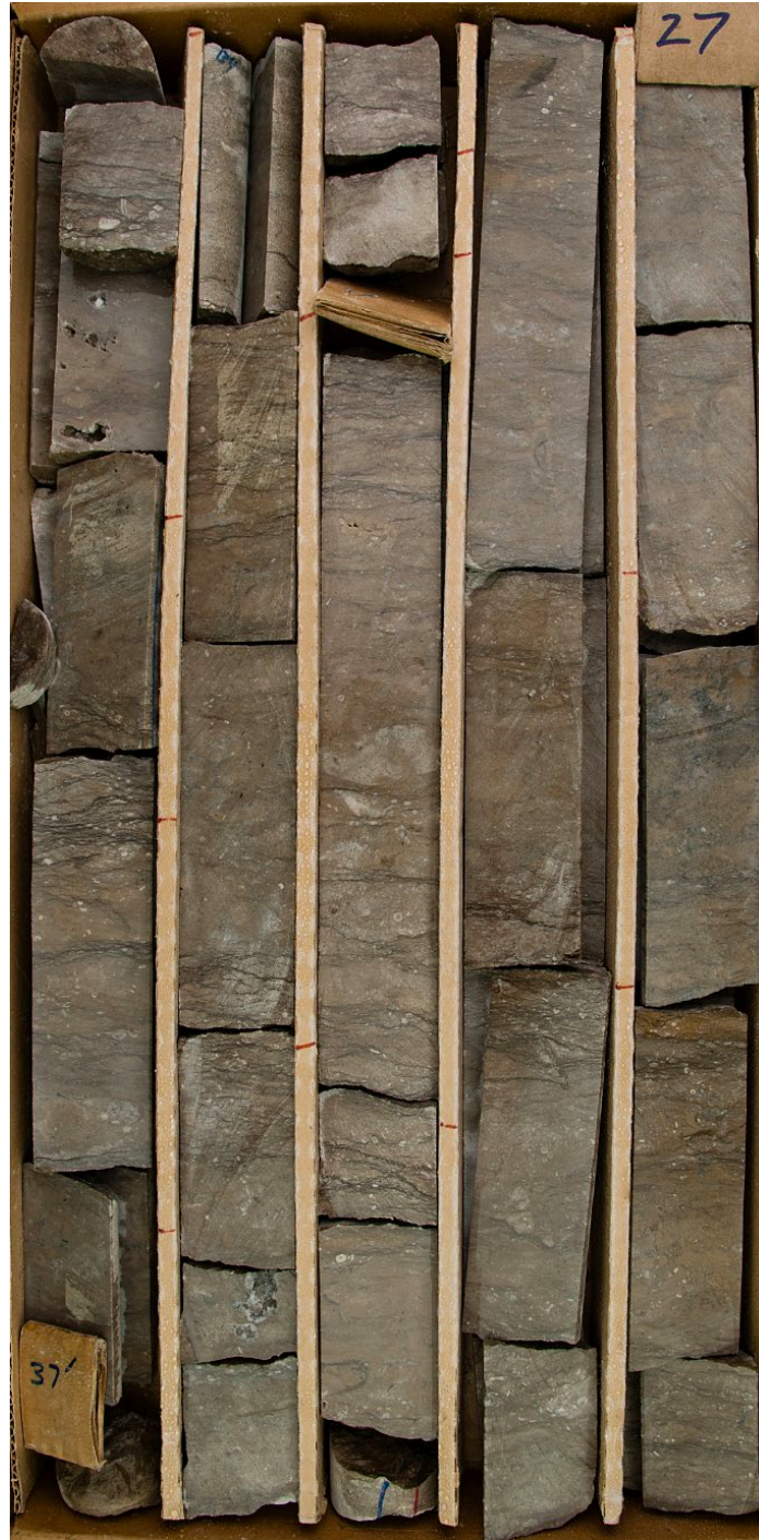
Figure 50. Swan Road, Box 2. Galena Formation dolomite wackestones facies with shale partings
