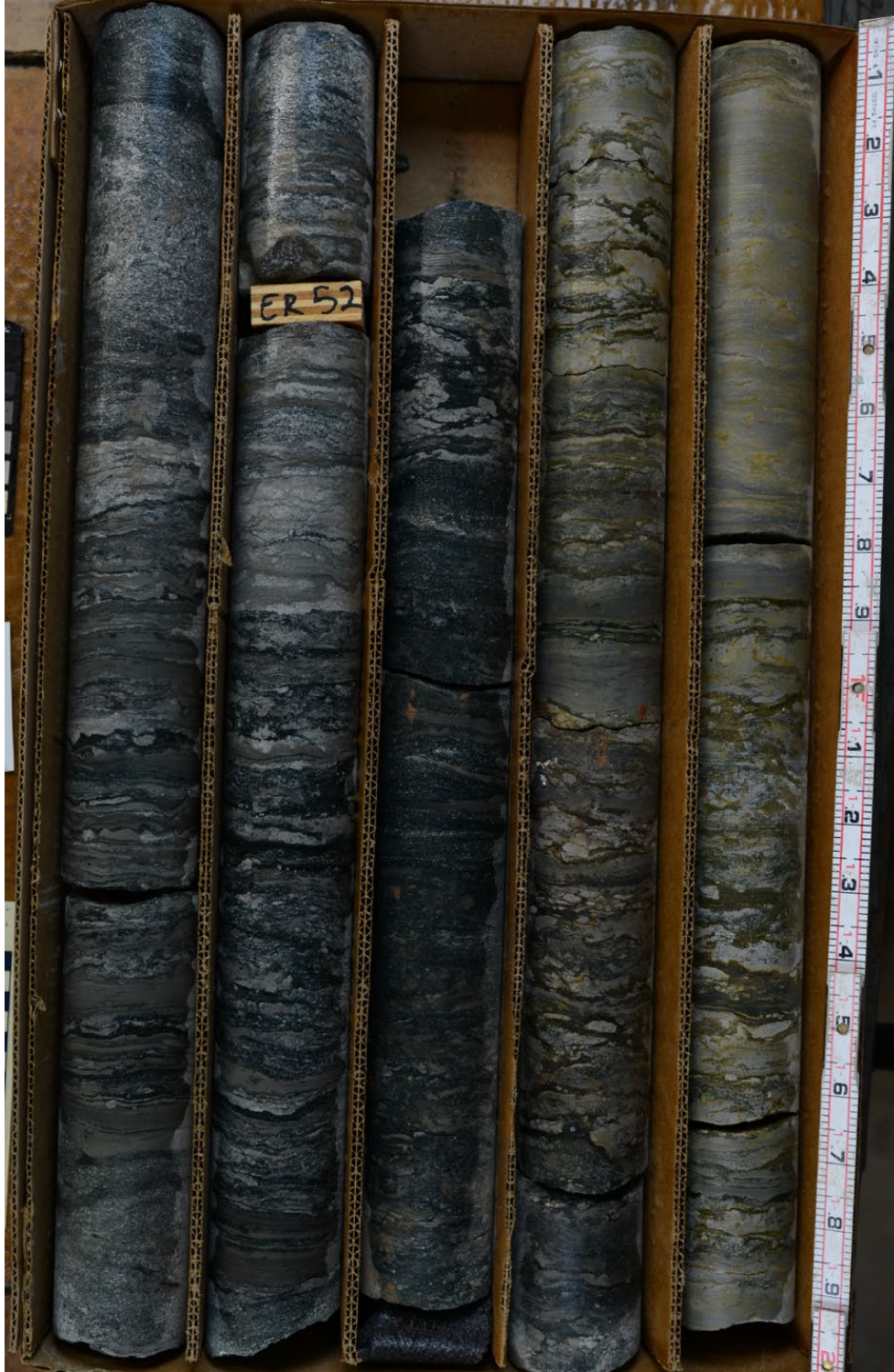
Figure 71. HBFA, Box 56. Eau Claire Formation bioturbated sandstone facies with interlaminated glauconitic fine-grained sand and gray mud with bioturbation, burrows, flame structures, and rip-up clasts.
