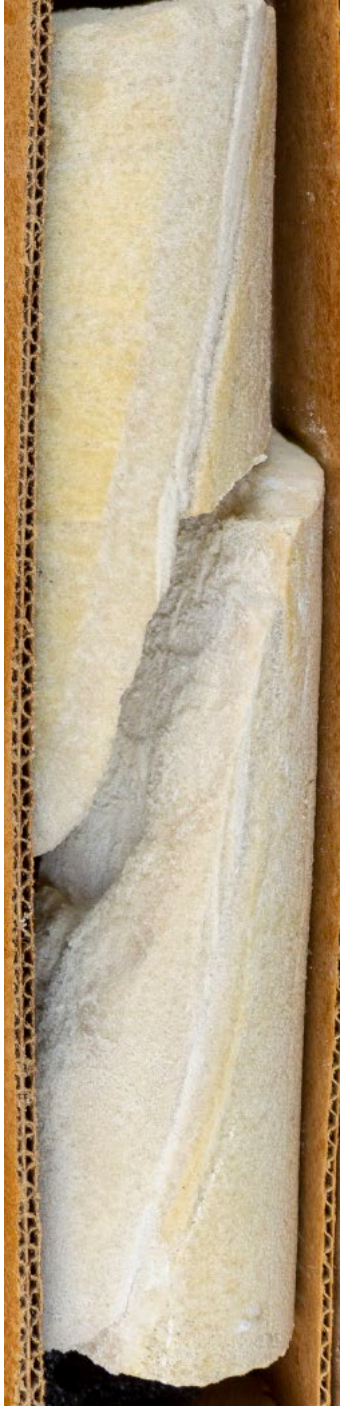
Figure 84. Mankowski, Box 7. Saint Peter Tonti Member massive sandstone facies with a high angle deformation band.
