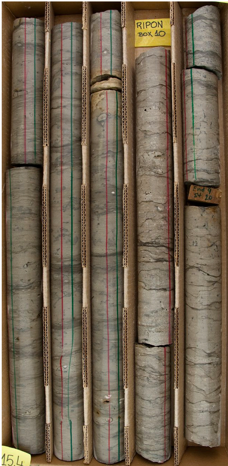
Figure 69. Ripon, Box 10. Sinnipee Group dolomite with shale partings and burrows.
