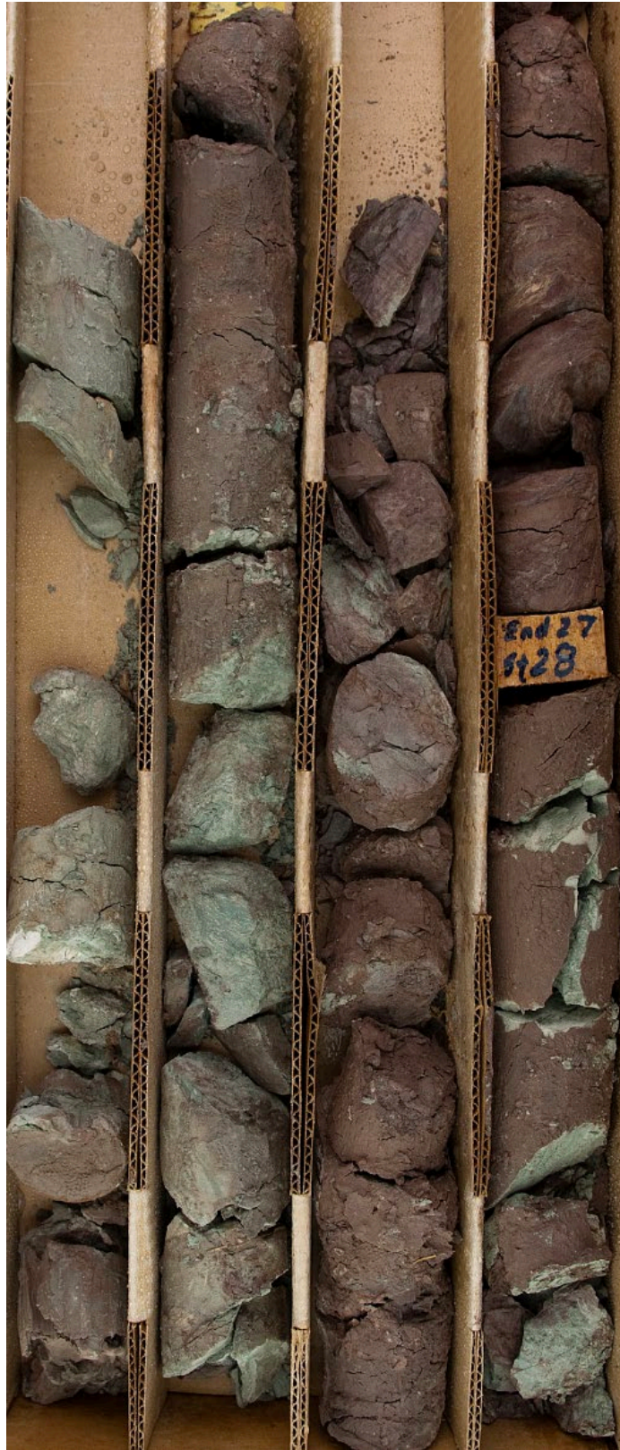
Figure 65. Ripon, Box 23. Lower Readstown Member soft sediment deformed strata facies.
