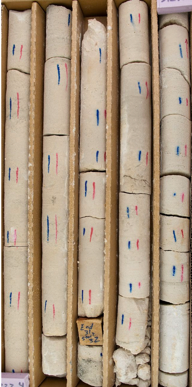
Figure 58. Rosendale, Box 30. Jordan Formation massive and cross-stratified sandstone facies.
