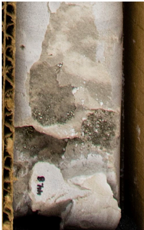
Figure 40. Buchda Quarry, Box 28. Millimeter-scale sulfide mineralization in vug of Shakopee Formation.
