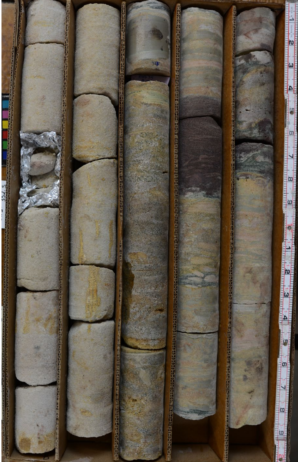
Figure 73. HBFA, Box 39. Wonewoc-Tunnel City sharp contact in the upper third column.
