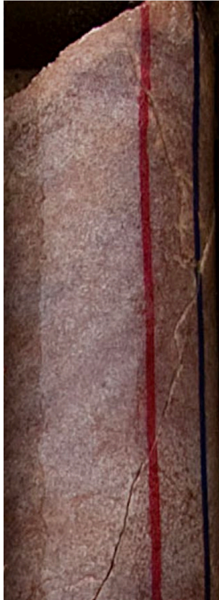
Figure 53. Highway T, Box 35. Fine grained red granite Precambrian basement.
