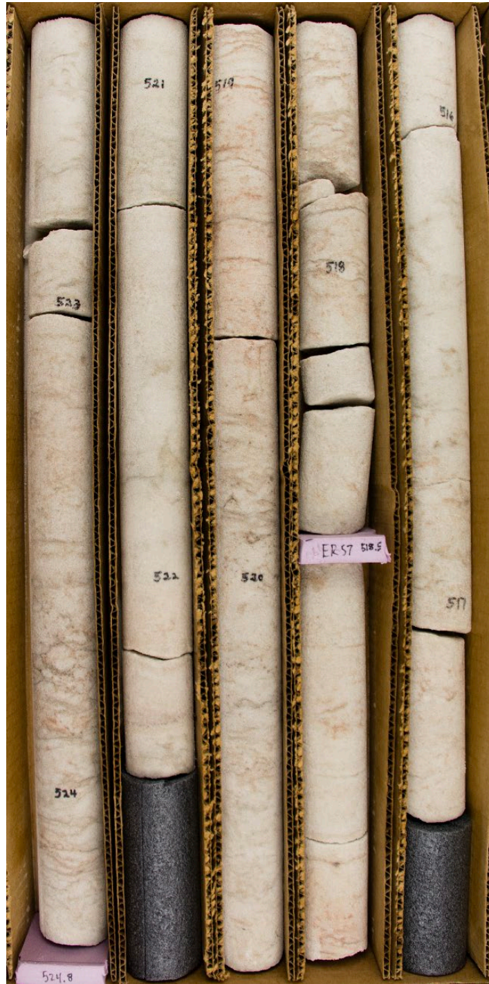
Figure 24. Keel, Box 51. Eau Claire fine sandstone with shale partings and bioturbation.
