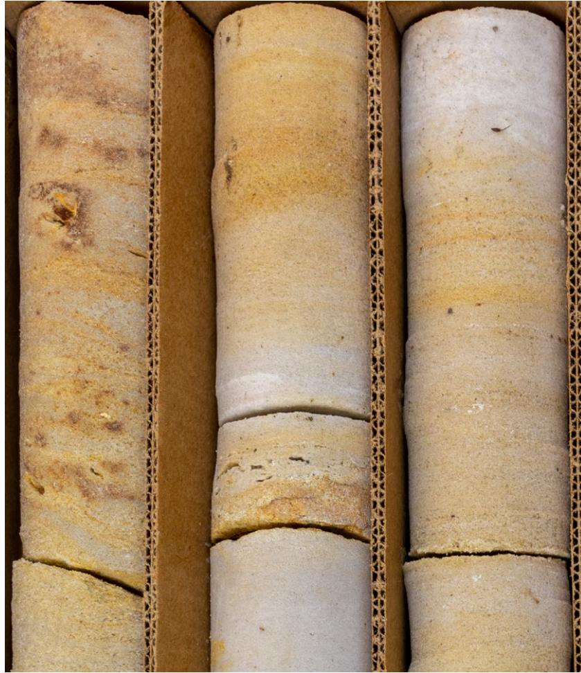
Figure 78. Mankowski, Box 17. Trempealeau Group Jordan Formation cross-stratified sandstone with iron staining and brachiopod shaped vugs.
