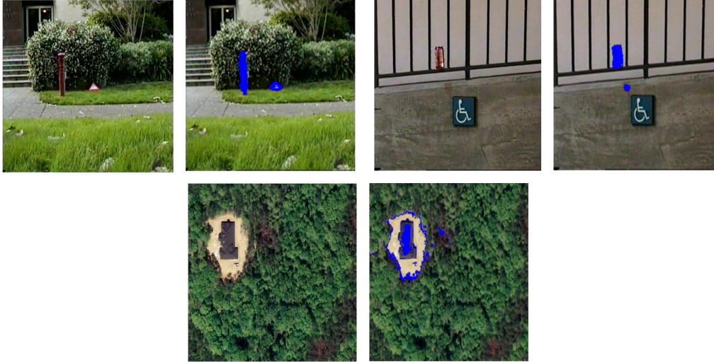
Figure 1: Results of the cluster based saliency method. The images on the left are the original images, and the ones on the right display the salient object occluded by an opaque patch.
