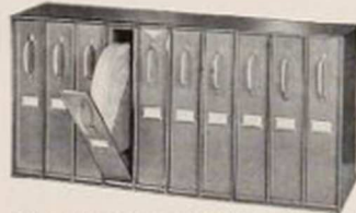
"ST" Series—Individual compartments for either one or two reels with a double wall air chamber between each compartment. Separate handle, index card and holder makes labeling easy. Stocked in 5, 6, 8, 10 and 12 compartment sections for all size reels.
