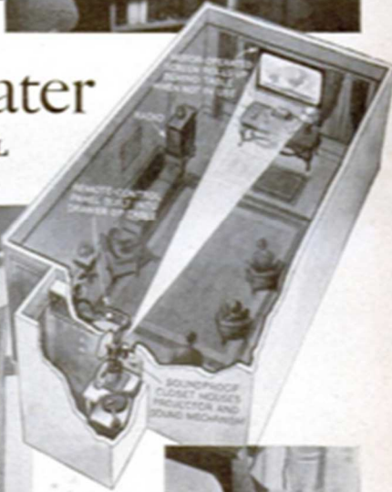
How the remote-controlled theater is arranged. The projection booth is a closet soundproofed with old bedding
