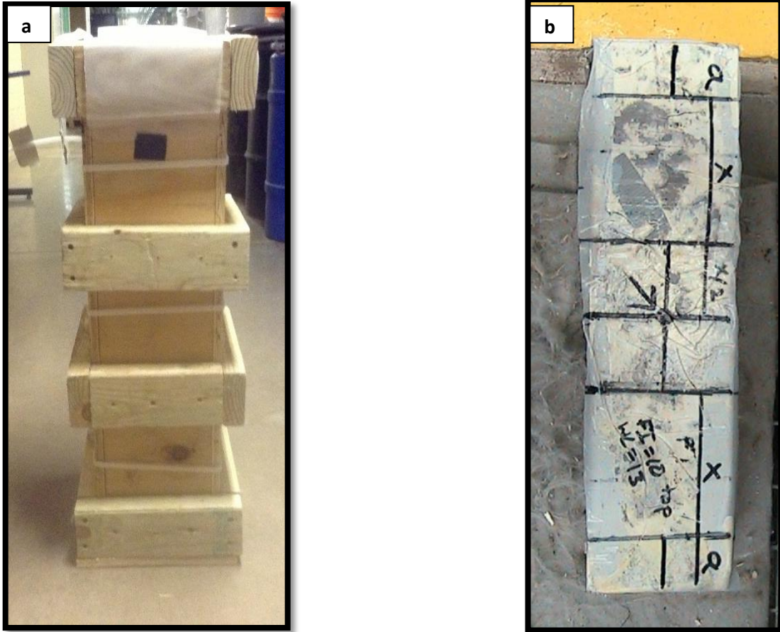
Figure 3.10 Picture of Beam Mold (a); Beam PSFB (b) after Injection
