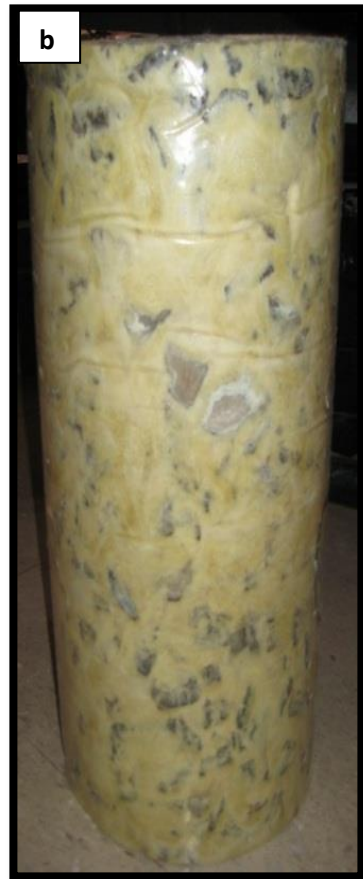
Figure 3.9 Cylindrical Mold (a), Cylindrical PSB (b) after Injection
