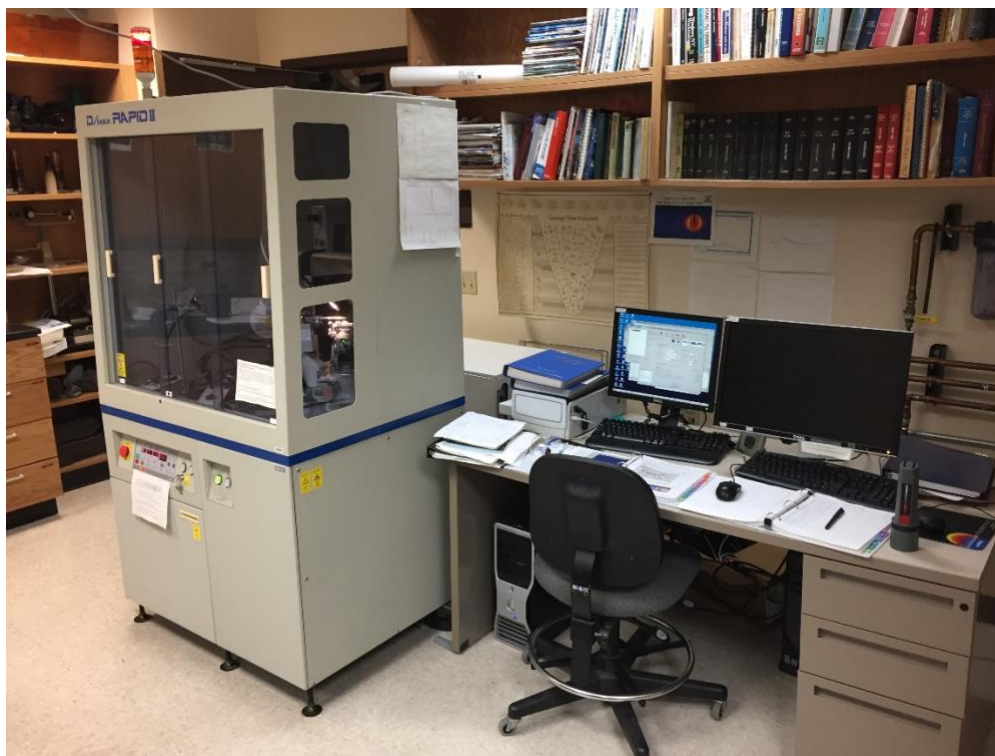
Figure 2-30 Rigaku D/Max Rapid II diffractometer used for X-ray diffraction analysis
