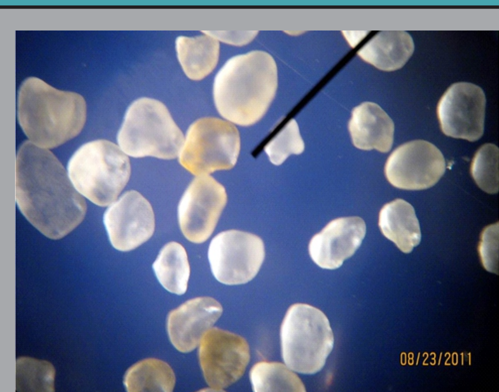
Figure 2. Frac sand grains (largest grains are 0.8 mm in diameter). Mining companies typically want sandstone containing strong, well rounded quartz grains between 0.2 and 0.8 mm diameter. From Kent M. Syverson.
