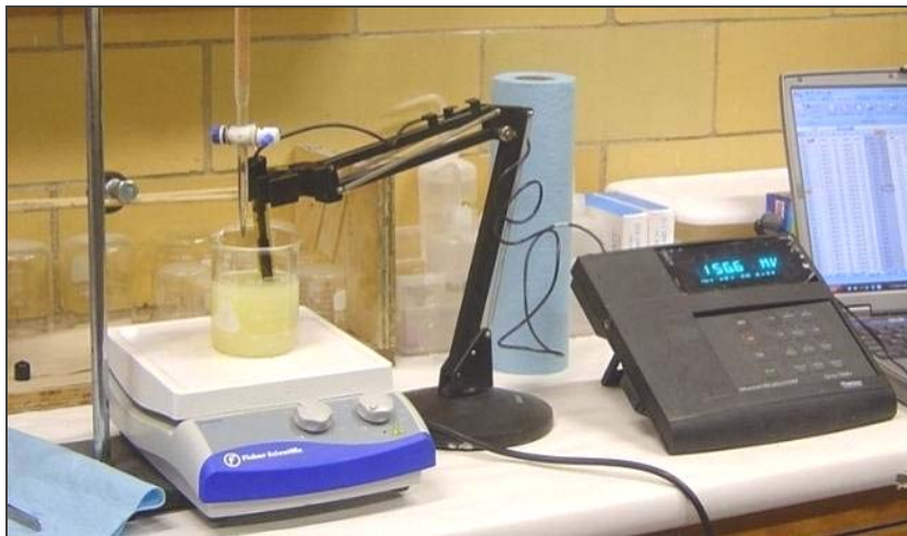
Figure 2.7: Testing set-up for measuring chloride ion content.
