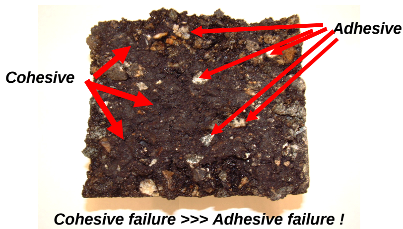
Figure 3.19 TSR Failure Surface of Asphalt Mixtures
