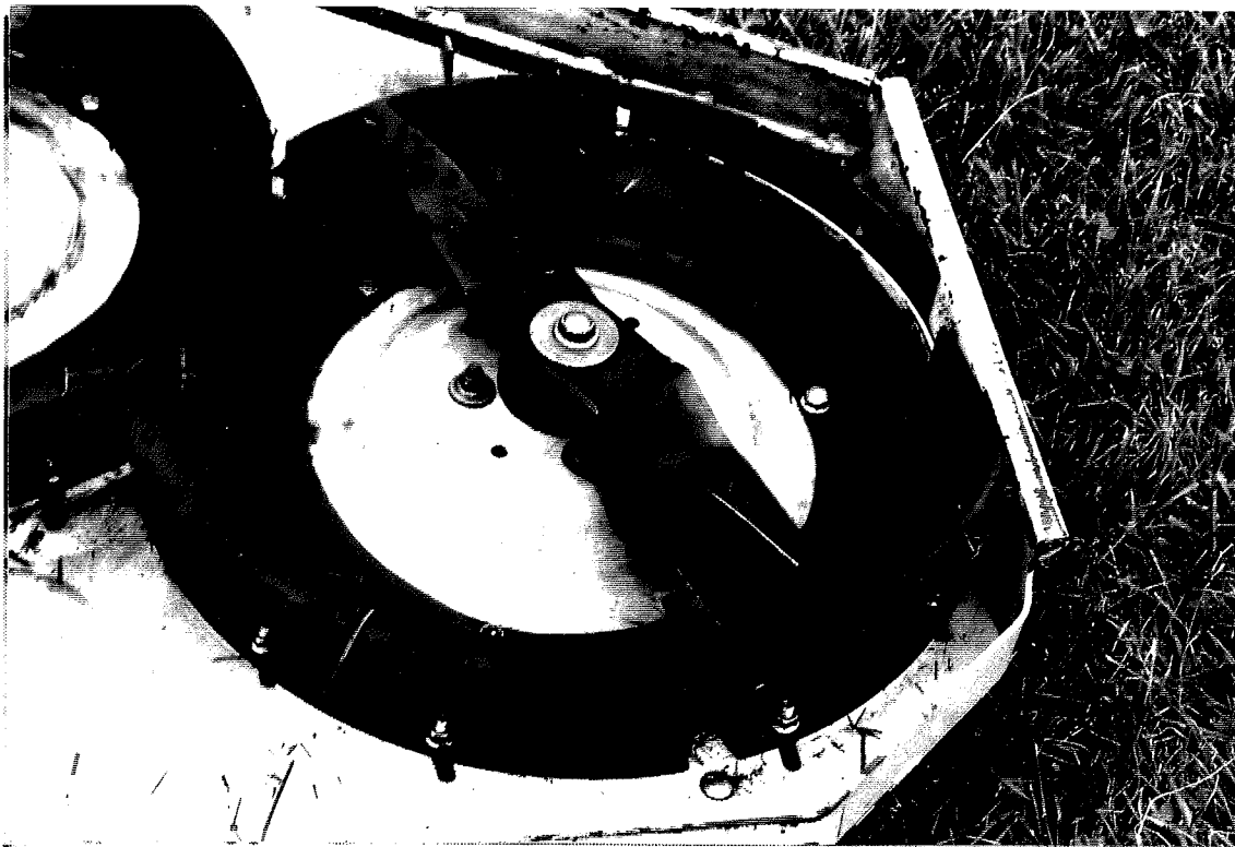
Figure 4.3 Close-up of left cutting chamber, with adjustable rear skirt in foreground.
