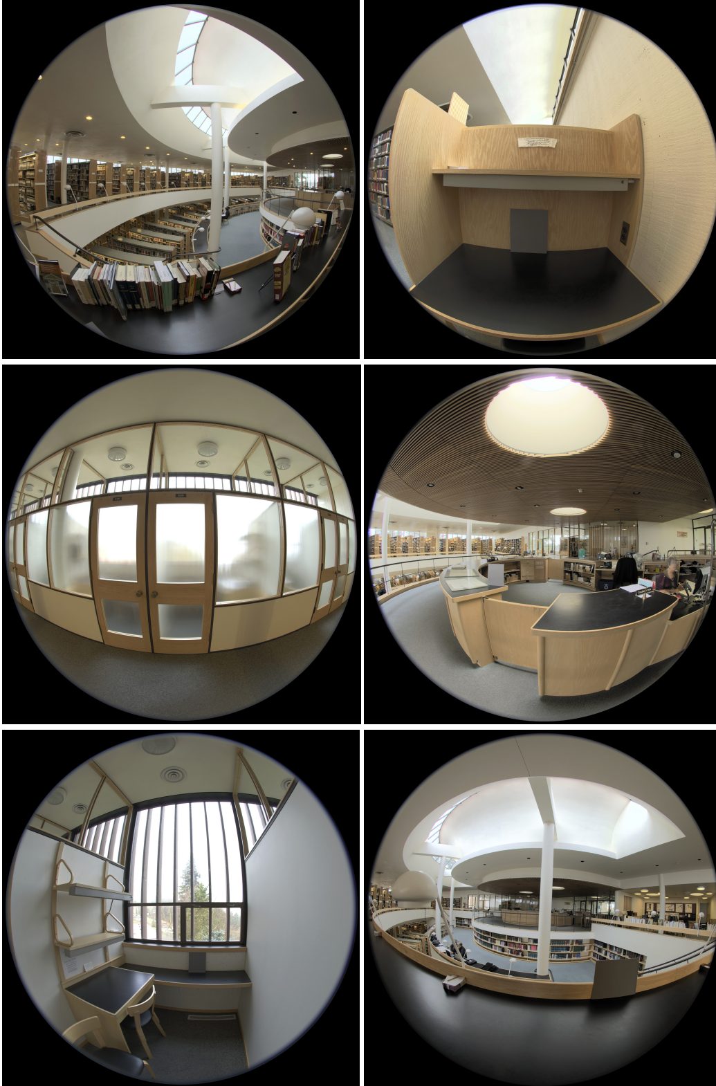
Fig. 7.1: Mt. Angel Abby library by Alvar Alto. Daylight sources are often hidden from direct view. The oblique surfaces create a soft transition between the light source and the interior surfaces. There are a variety of seating areas with different levels of daylight for the visitors to choose from.
