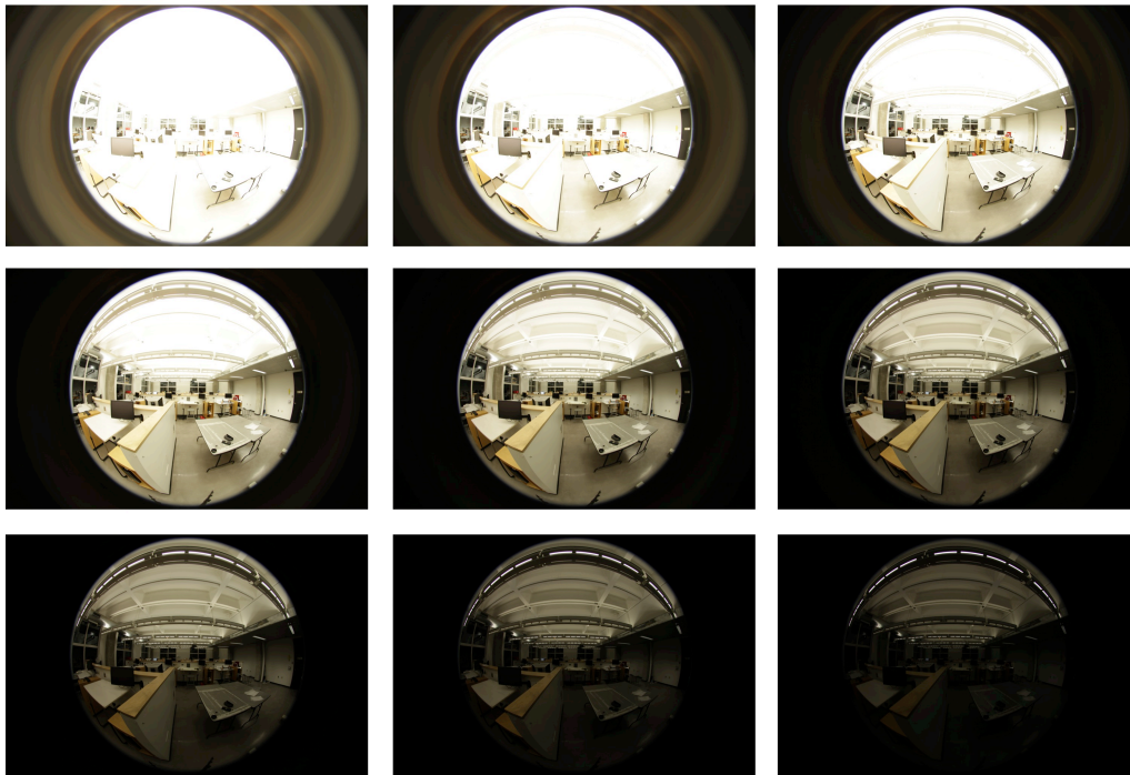
Fig. 6.4: Exposure bracketed images captured at night to compute an HDR image
