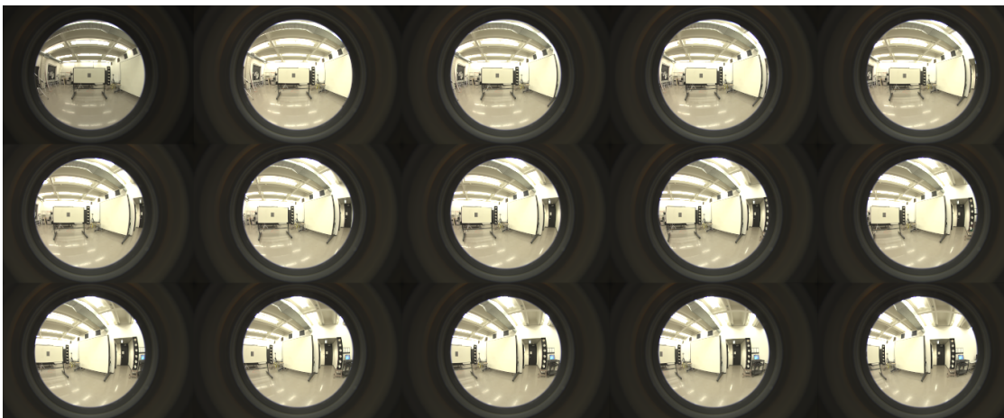
Fig. 4.7: HDR images of the target (grey card) at 5-degree increments.
