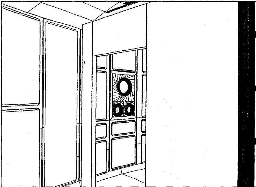
Figure 5.2.6.2.7-1. A limited hygiene facility services the exercise area and alleviates the need for the crew to translate to the lower level.
