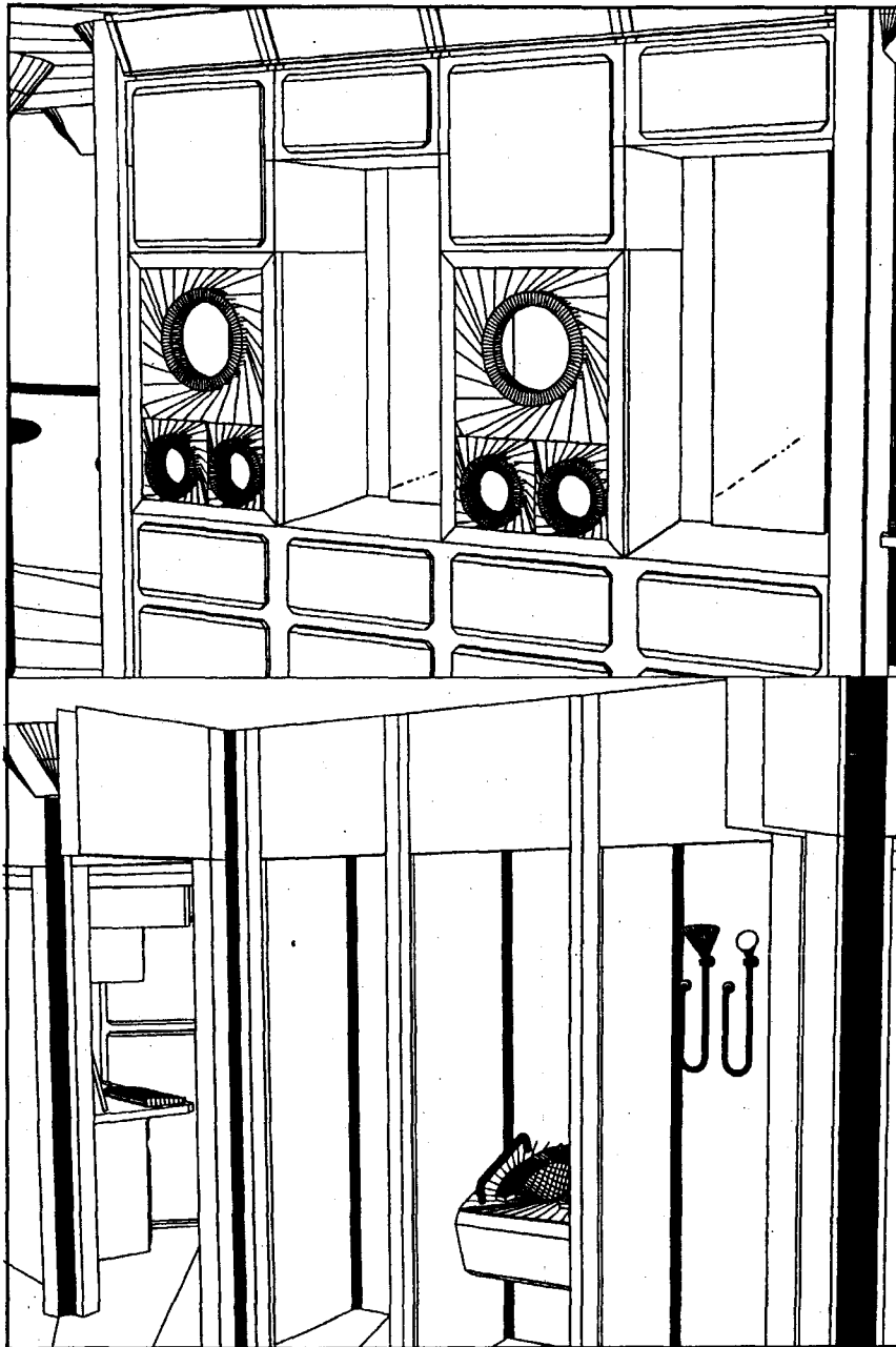
Figure 5.2.6.1.4-1 (a and b). Hygiene facility provides hand/face/eye washing capability along with full body cleansing.
