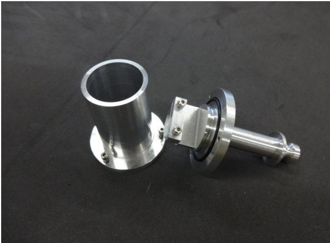
FIGURE 35 FABRICATED TENSILE TESTER WITH SATURATION CHAMBER
