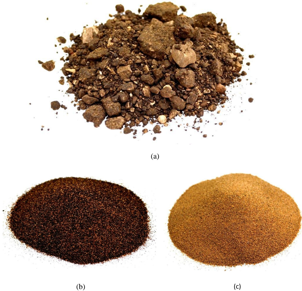
Figure 4 RAP material: (a) Un-sieved RAP material, (b) R #100 RAP, and (c) Burned R #100
