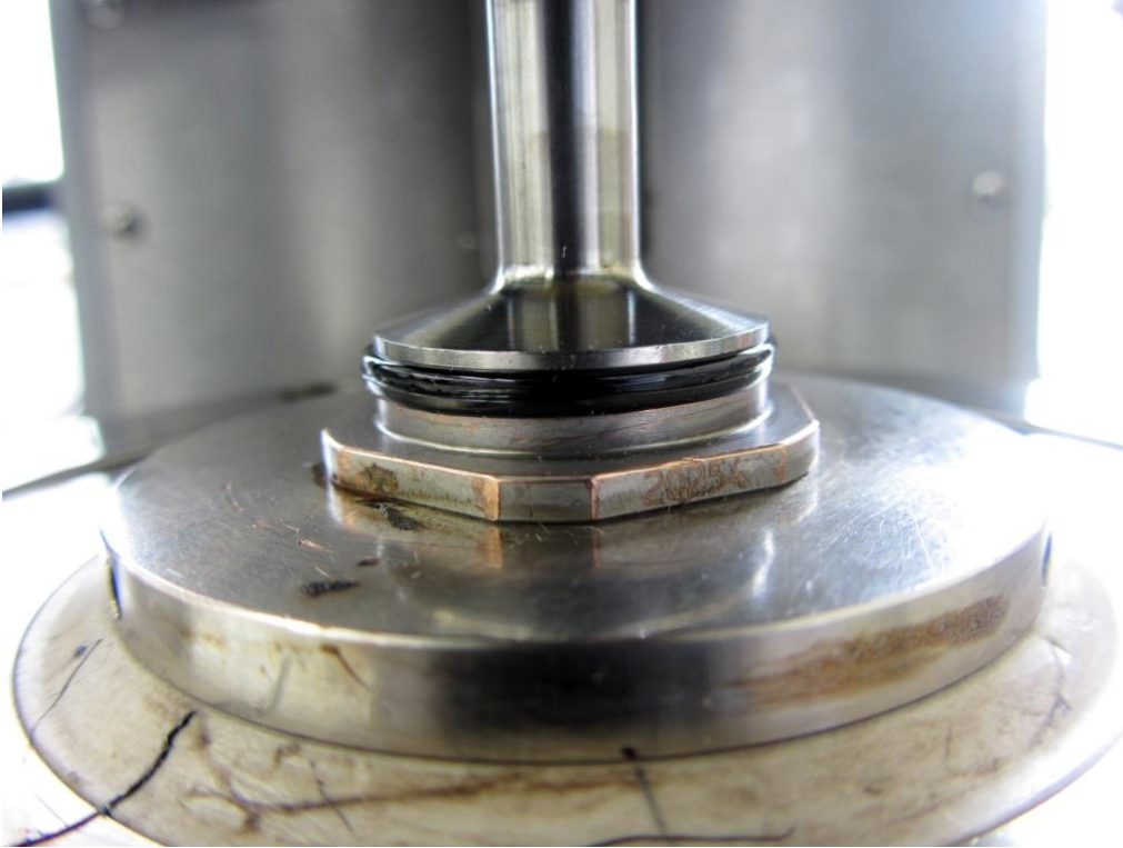
Figure 24 Asphalt binder sandwich conditioning in the DSR
