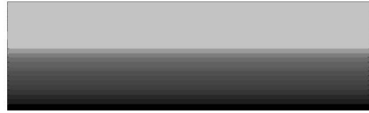
b) Blended binder regions start forming due to diffusion of fresh binder in the aged binder layer.
