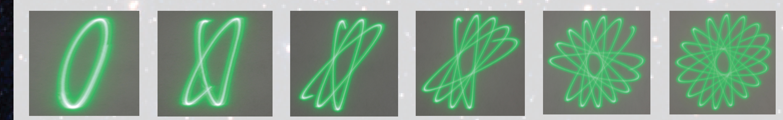
These photographs show a 40:41 ratio and the effect of the phase difference. Imaged at different shutter speeds.
