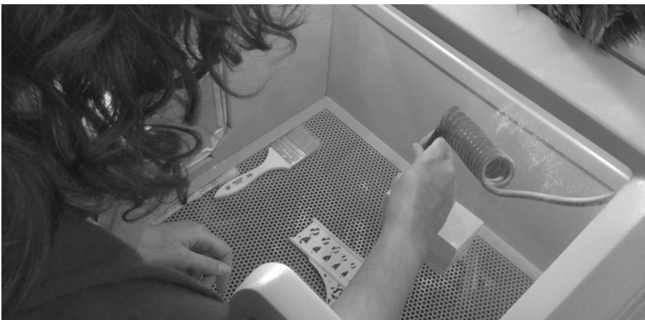
The final traces of powder are removed during the postprocessing phase. Photo by Austin Pontius.
