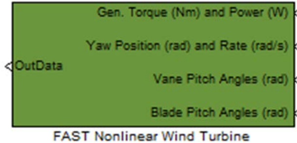
Fig. 7.3. Simulink Interface of FAST including Vertical Vane Pitch Control.
