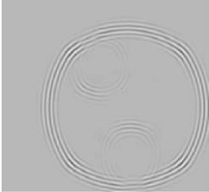
Figure 1.17 Propagating wave in composite plate at 0.16 milliseconds [30].
