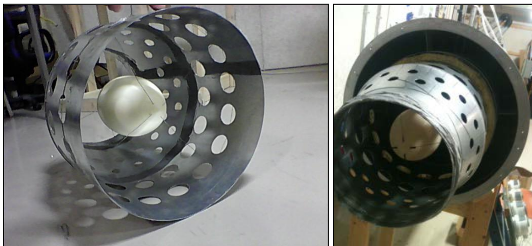
Figure 3.11 Streamlined body mounted in the test-section.
