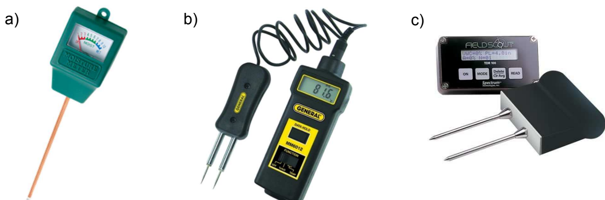
Figure 1.2. Commercially available electromagnetic soil moisture sensors. a) Resistance sensor (Amazon Soil Moisture Meter). b) Capacitance sensor (General® Moisture Meter). c) TDR sensor (FieldScout® TDR Moisture Meter).
