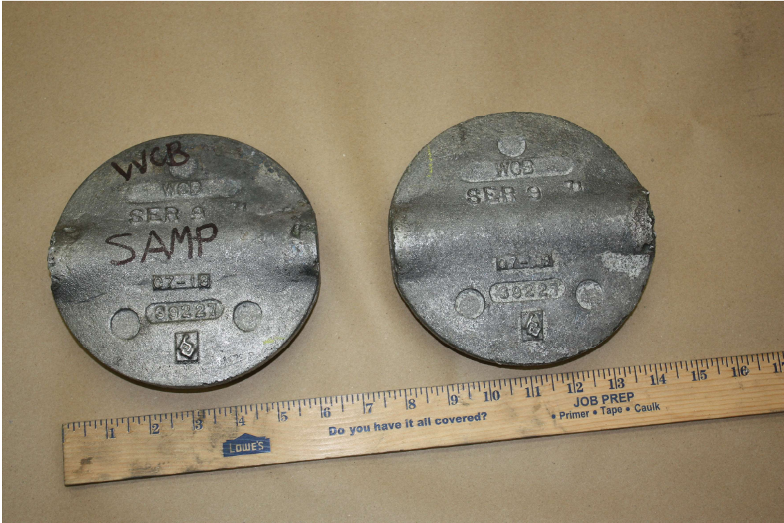
Figure 3.5: Surface alloyed butterfly valve prototypes cast at Badger Alloys. Ni, Cr, Fe-Mn and Fe-Si were used as alloying powders. REFCOHOL 1010 and Sodium Polyacrylate were used as separate binders.
