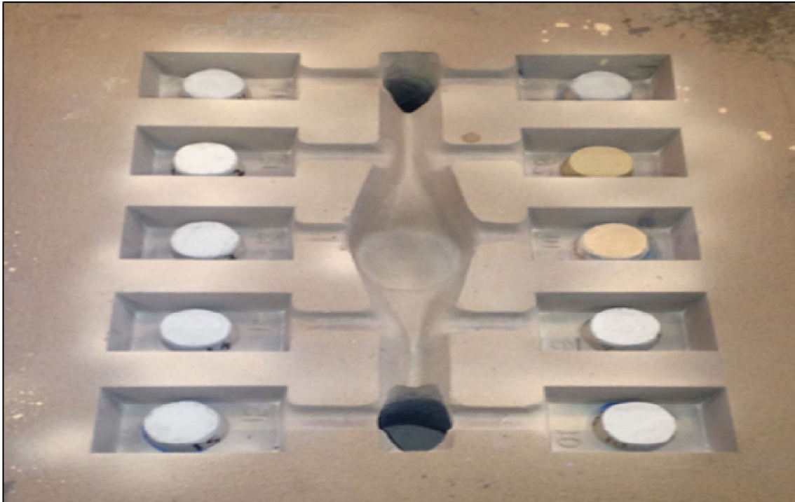
Figure 3.3: Mold and slurry coated sand cores for castings made at Maynard Steel.
