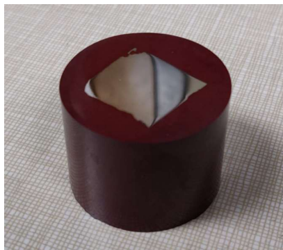
Figure 3.11: Surface alloyed UWM Foundry Lab sample R2 mounted in phenolformaldehyde compound.
