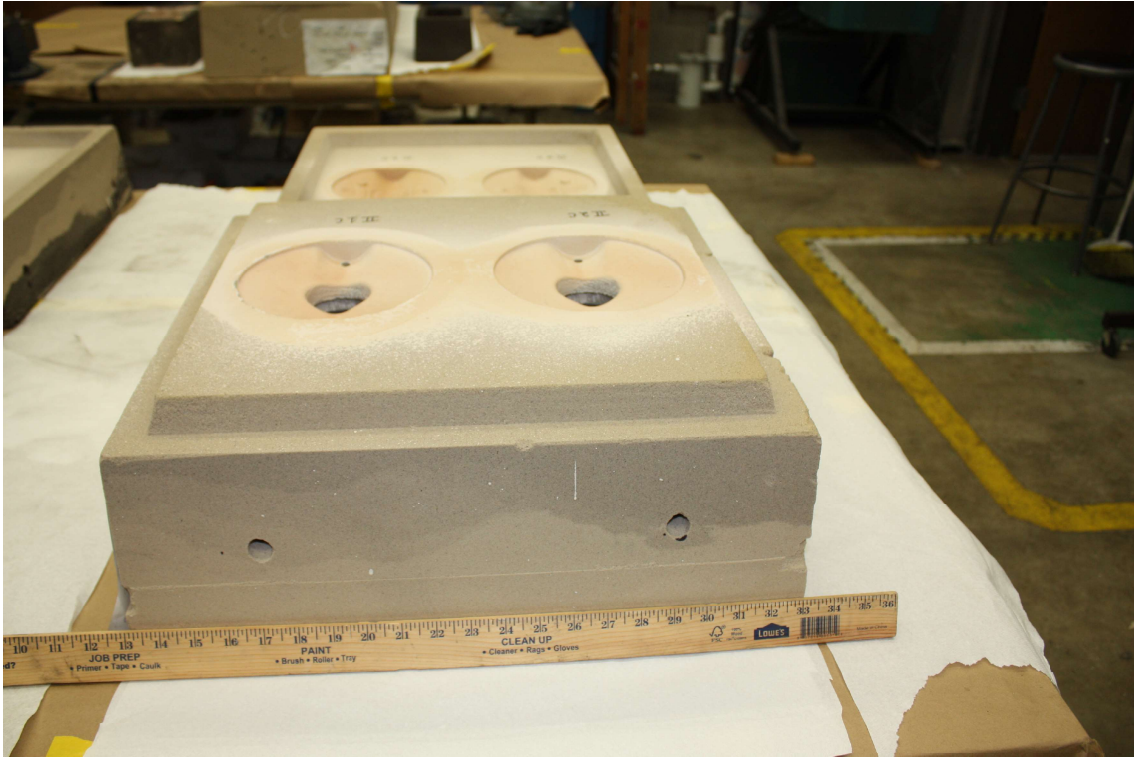
Figure 3.6: Molds for butterfly valve made at Badger Alloys for casting an industrial surface alloyed prototype.
