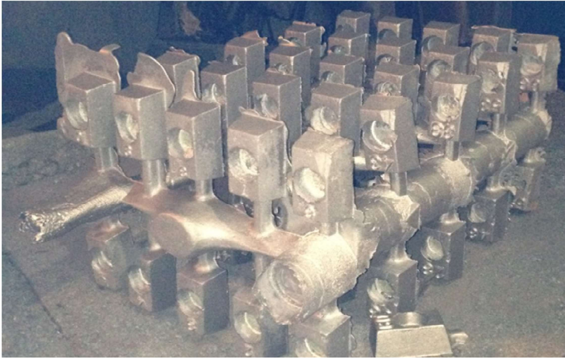
Figure 3.4: 50 units of 10-lbs castings poured at Maynard Steel.
