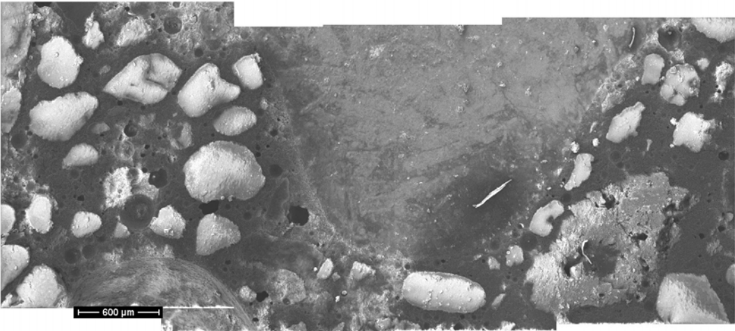
Figure IV.2 – Hardened Air Void Distribution of Hw53 Sample
