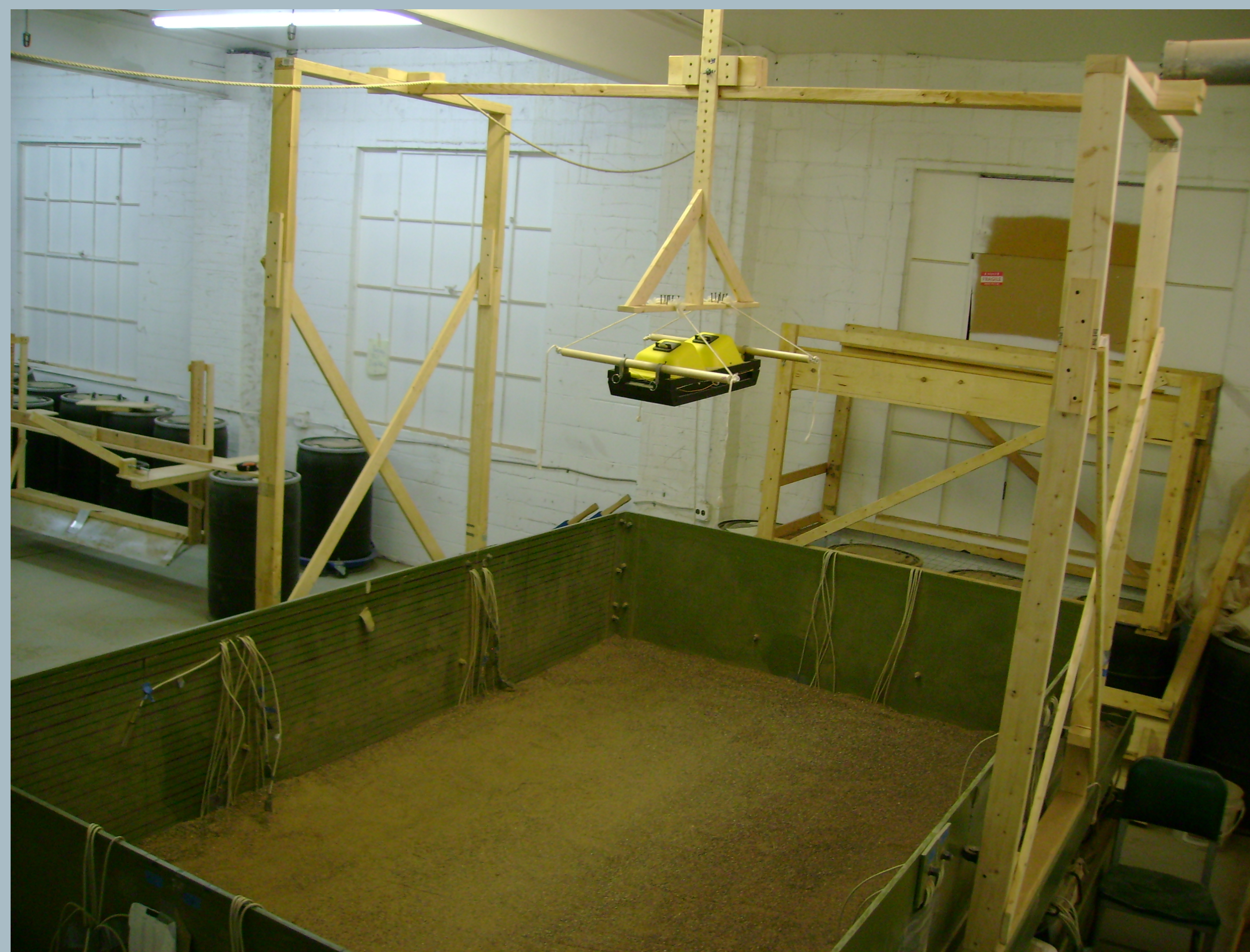
Figure 1: Multi-frequency GPR data were acquired after each new soil layer was added. This figure shows data acquisition with the 500 MHz antennas. GPR surveys were also acquired over a 1.5-m by 1.5-m steel plate placed in the tank to generate the maximum reflection amplitudes needed to calibrate the reflections from the soil surface.
