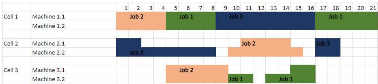
Figure 19: Detailed schedule for a 3-job, 3-machine, 3-operation instance with two machines per cell, three machine breakdowns, and processing time variability
