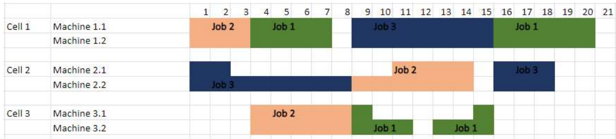
Figure 18: Detailed schedule for a 3-job, 3-machine, 3-operation instance with two machines per cell and three machine breakdowns
