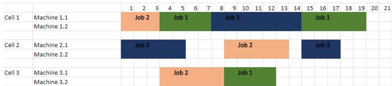
Figure 17: Detailed schedule for a 3-job, 3-machine, 3-operation instance with two machines per cell and no machine breakdowns (same as Figure 2)
