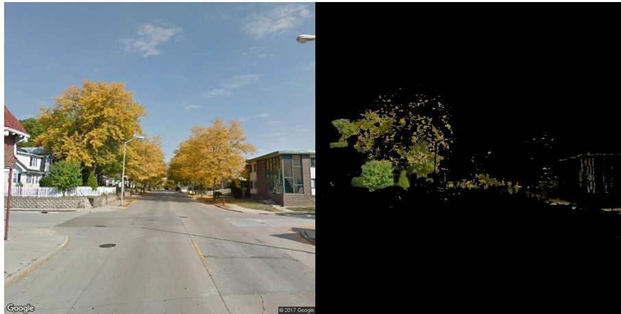
Figure 9: The image processing filter fails to detect yellow-colored vegetation image components. Notice also false positive detection of green components of a building. Left: Original RGB Image. Right: Masked image that has been produced by a green vegetation detecting image processing filter [17, 6]
