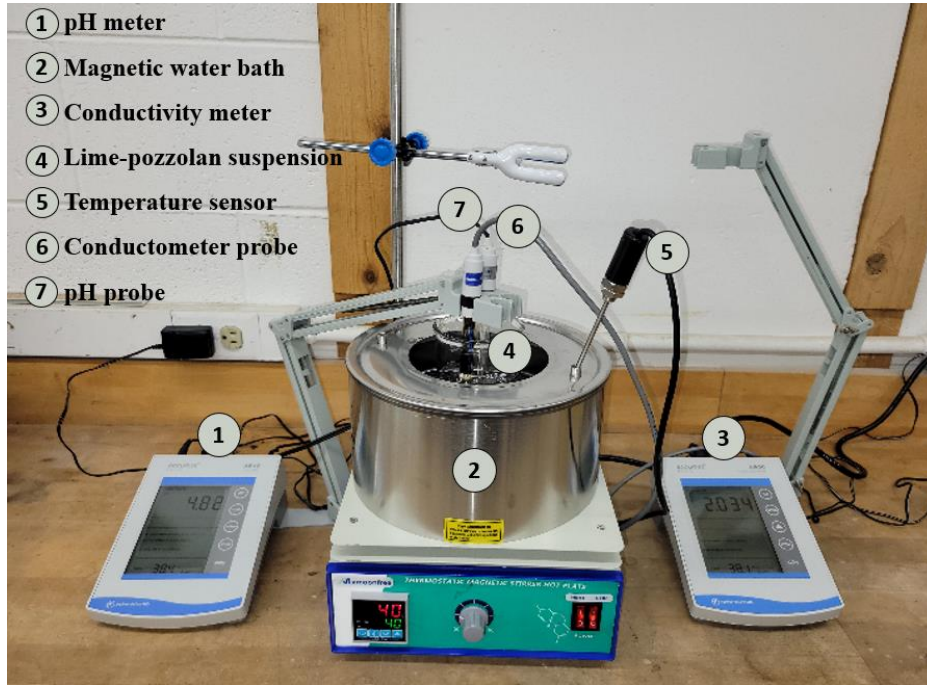
Figure 3-3: Electrical conductivity and pH test setup.
