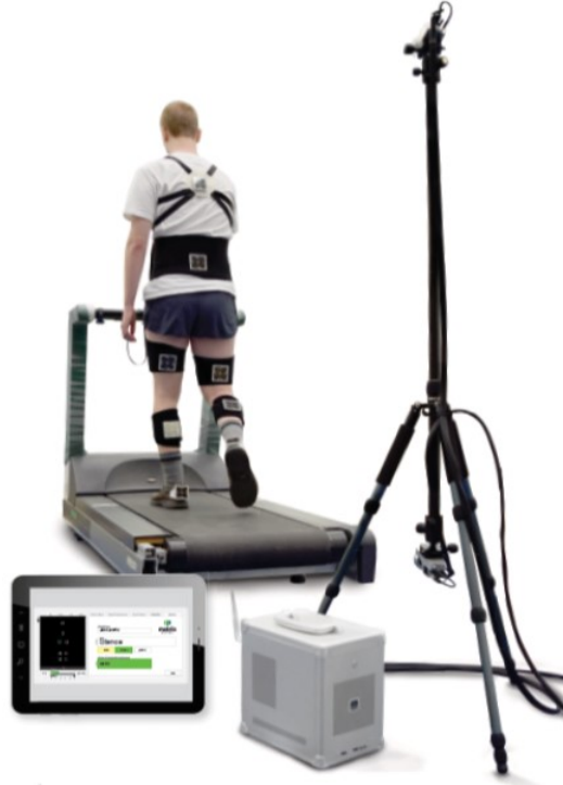
Figure 5: Measurement apparatus for collecting gait movement data. The apparatus utilizes two cameras to capture a larger field of view and operates with eight markers, a single marker placed per body segment.
