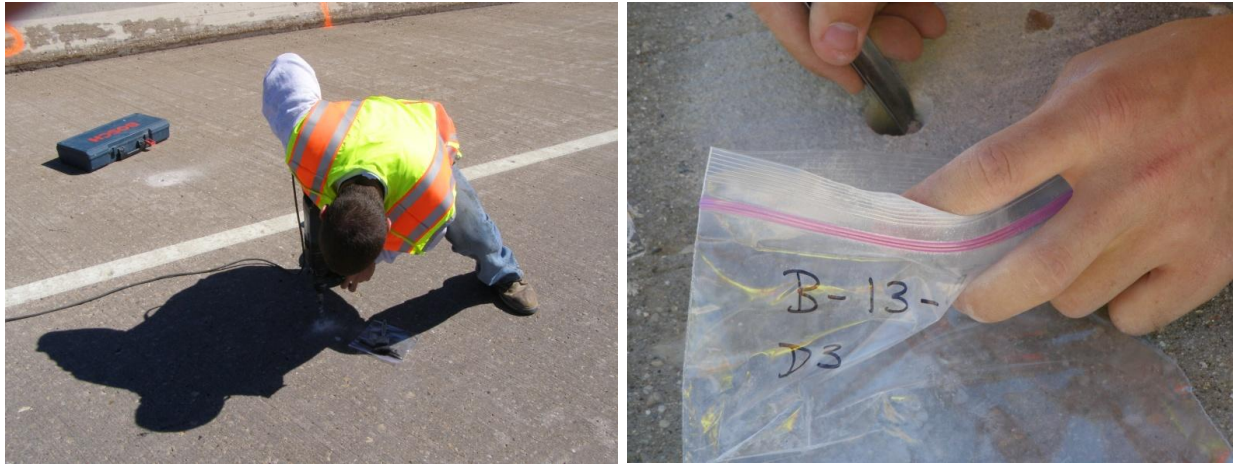
Figure 4.2 Extraction of powder samples in the field.
