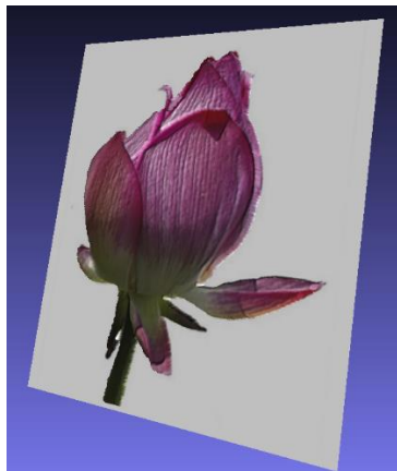
Figure 3.10: The output of a small flower image based on this algorithm, with added texture. The range between the foreground and background is more obvious than the internal features, a trait typically resulting from 2D algorithms.
