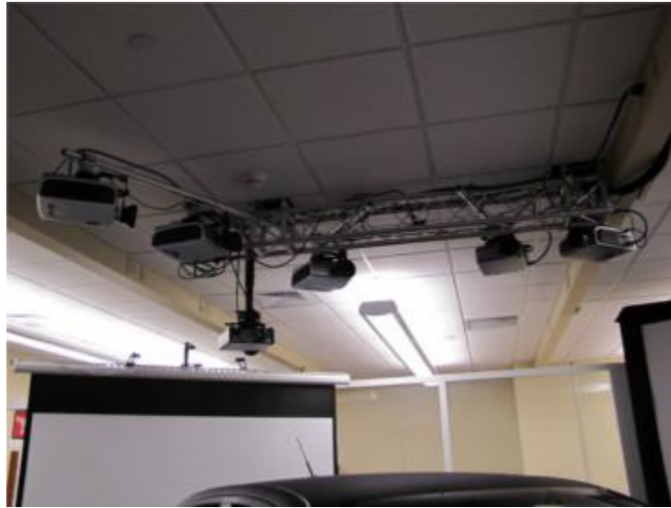
Figure 4: Projectors Responsible for Producing the Driving Environment (40)
