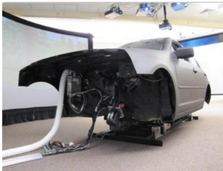
Figure 5: Ford Fusion Mounted on 1-Degree of Freedom Motion Platform (40)
