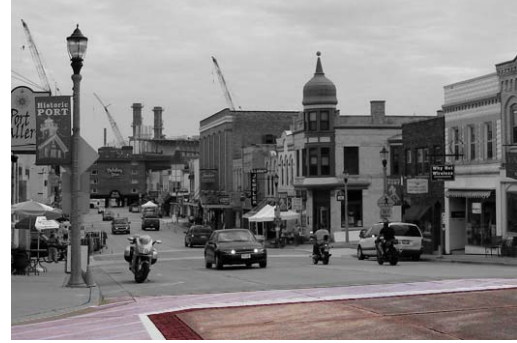
Variations in color and material to define intersection and cross-walk Port Washington, Wisconsin
